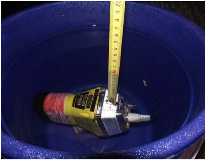
Figure 9.1 – View of the EUT in the water during the Leakage Test
