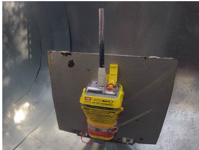
Figure 17.7 - View of EUT (MT603G) upon completion of inadvertent activation test
