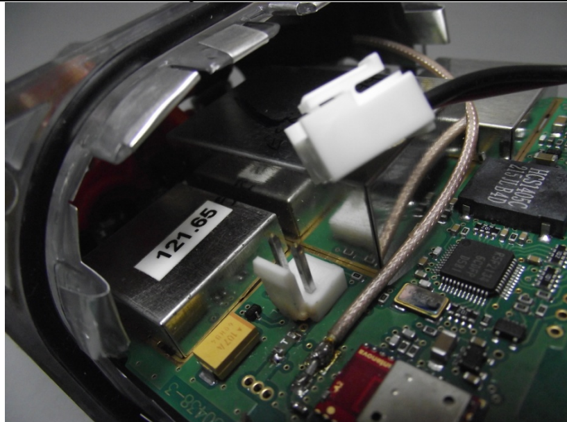
Figure 19.3 - View of the PCB upon completion of the humidity test
