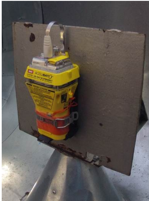
Figure 17.1 – EUT (MT603G) mounted on the rotatable support before test.
