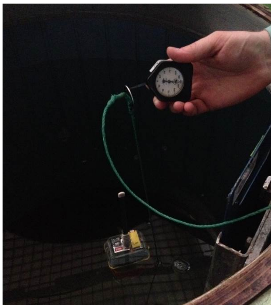
Figure 16.3 – Measuring of buoyant force
