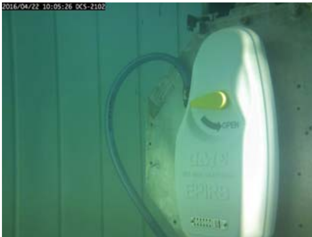
Figure 15.1 – The satellite EPIRB automatically released at normal orientation after maintained at minimum storage temperature.
