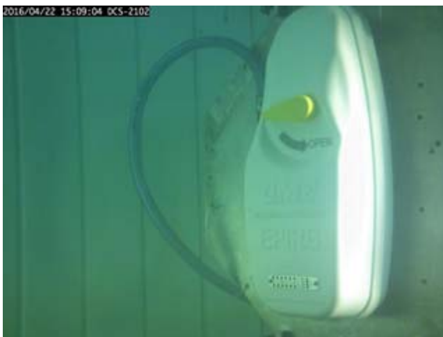
Figure 15.2 - The satellite EPIRB automatically released at normal orientation after maintained at maximum storage temperature.
