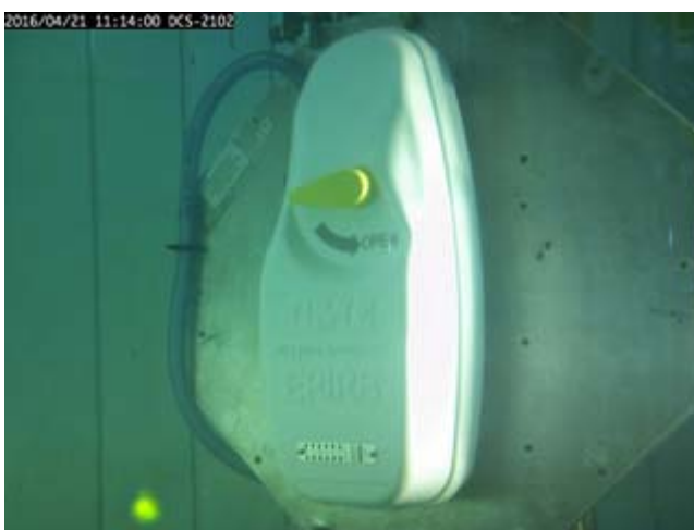
Figure 15.3 - The satellite EPIRB automatically released at normal orientation at ambient temperature.
