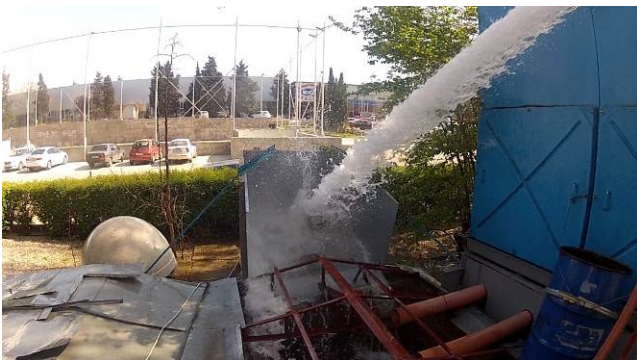
Figure 17.6 - The water strikes EUT (MT603FG) in an arc of 180°.
