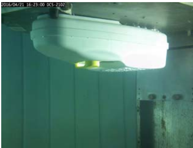
Figure 15.6 - The satellite EPIRB automatically released at Pitching 90° bow down orientation
