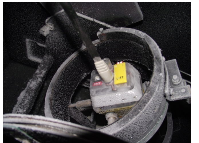
Figure 13.6 – View of the EUT upon completion of the low-duty cycle test at minimum temperature
