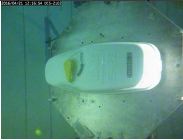
Figure 15.4 - The satellite EPIRB automatically released at Rolling 90° starboard orientation
