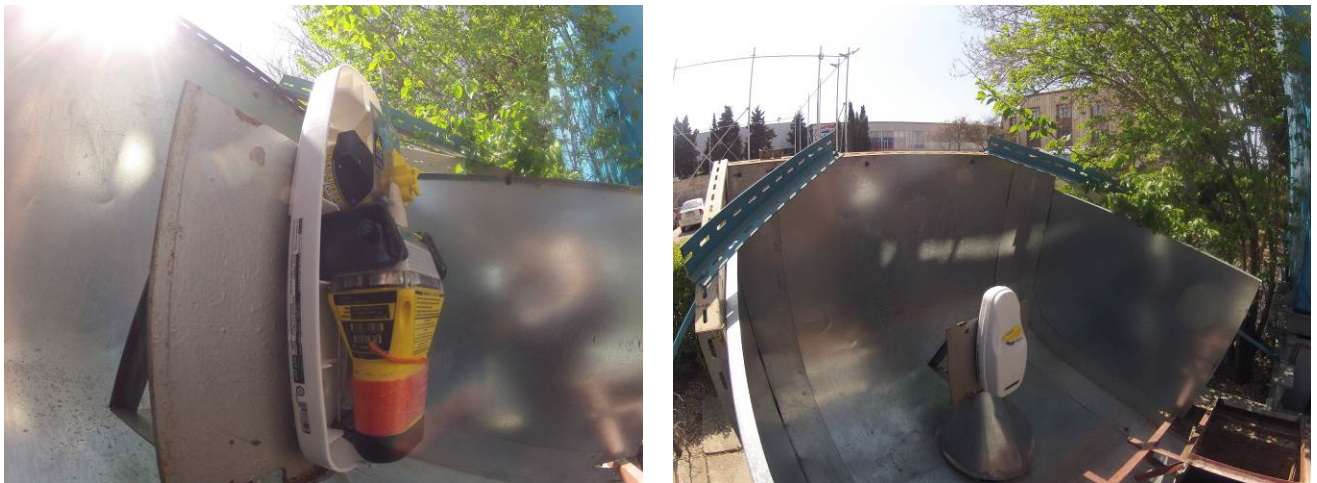
Figure 17.2 – EUT (MT603FG) mounted on the rotatable support before test.
