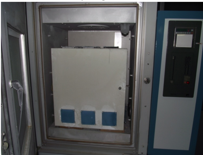
Figure 13.3 – General view of rotation and inclination device inside of the climatic chamber
