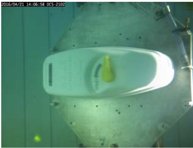
Figure 15.5 - The satellite EPIRB automatically released at Rolling 90° port orientation
