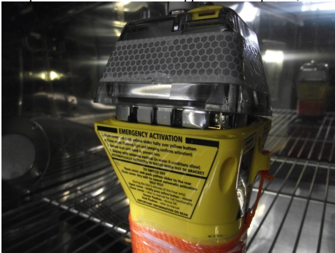
Figure 19.1 - View of the MT603FG with the opened housing before the humidity test
