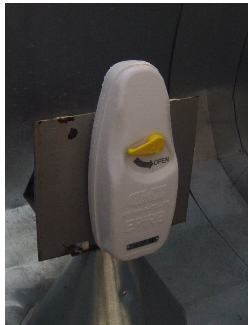
Figure 17.8 - View of EUT (MT603FG) upon completion of inadvertent activation test
