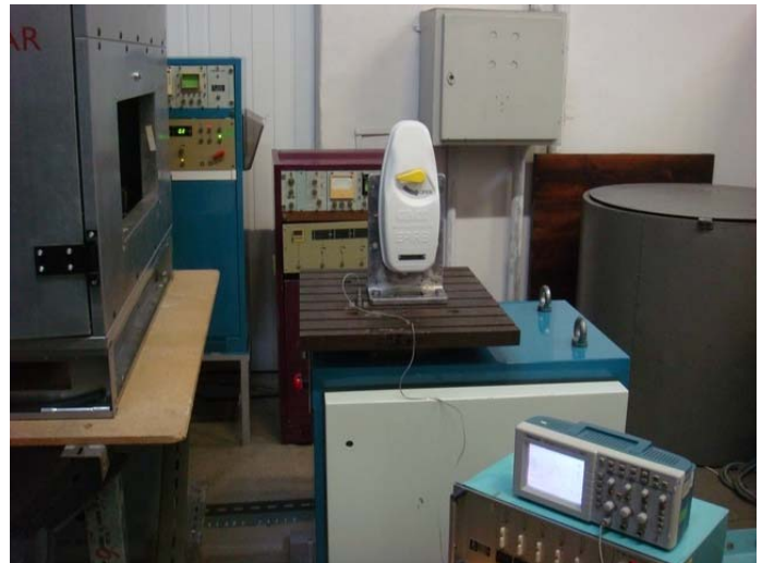
Figure 5.3 - Test Set-up. Vertical axis of the MT603FG
