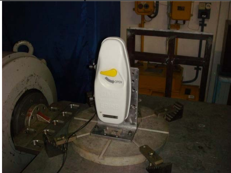
Figure 4.16 - General view of the horizontal Y vibration test (MT603FG)
