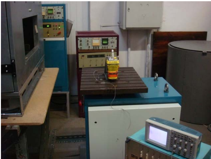
Figure 5.2 - Test Set-up. Vertical axis of the MT603G
