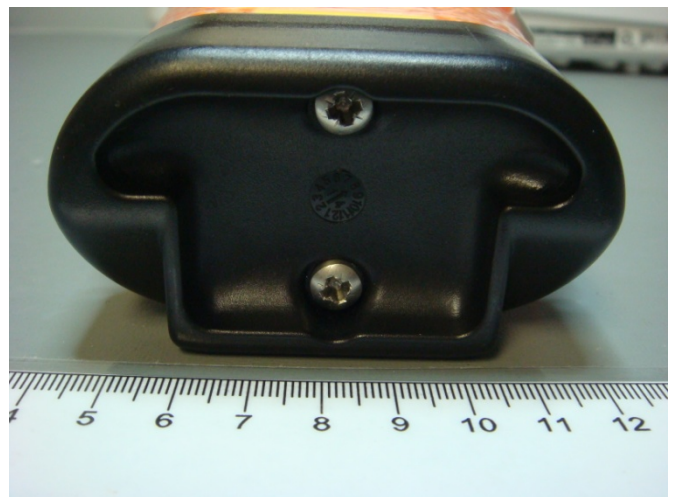
Figure 6.5 – View exterior inspection of the MT603FG upon completion of the salt fog test
