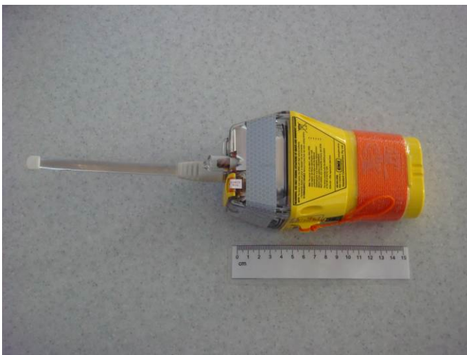
Figure 5.4 – View of the MT603G upon completion of the bump test
