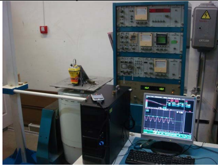
Figure 4.1 - General view of the test site vertical Z vibration (MT603G)
