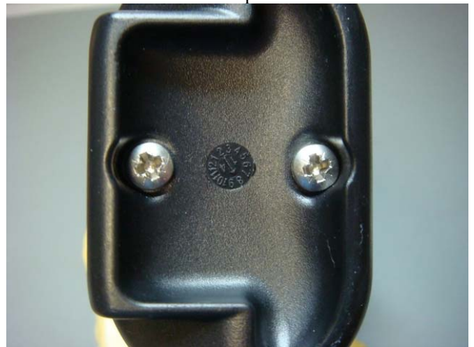
Figure 5.7 – View of the MT603FG upon completion of the bump test
