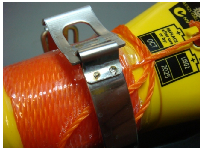
Figure 6.2 – View exterior inspection of the MT603G upon completion of the salt fog test
