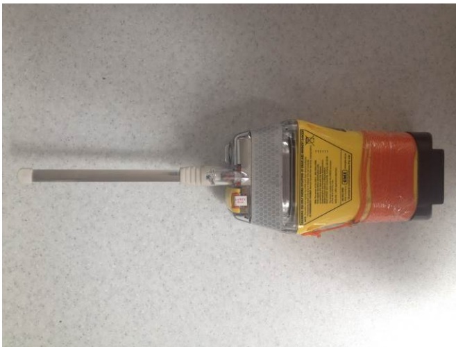
Figure 7.4 - View EUT upon completion of the drop test
