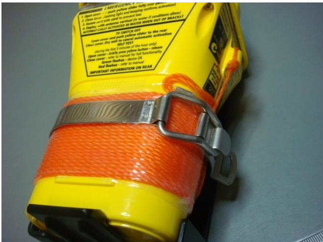
Figure 6.2 – View exterior inspection of the MT603G upon completion of the salt fog test
