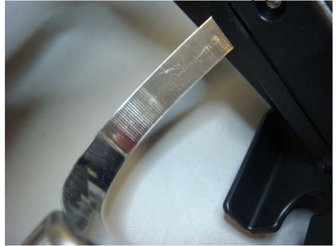
Figure 5.8 – View of the MRH (MT603FG) upon completion of the bump test
