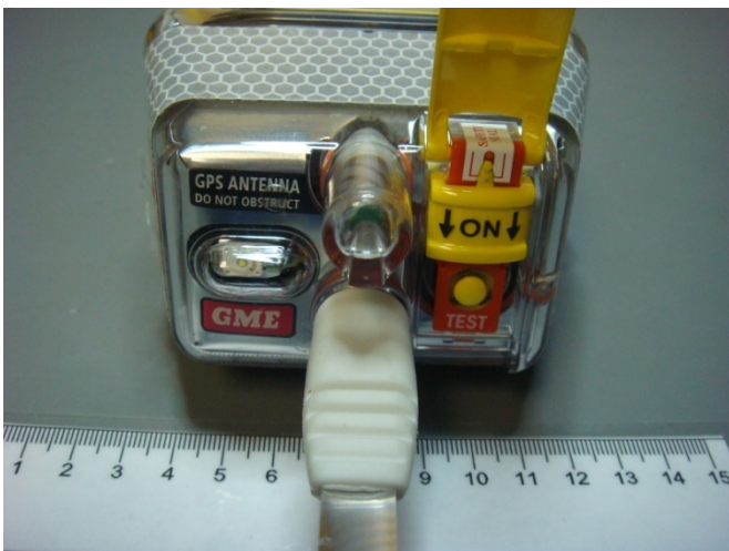
Figure 6.5 – View exterior inspection of the MT603FG upon completion of the salt fog test
