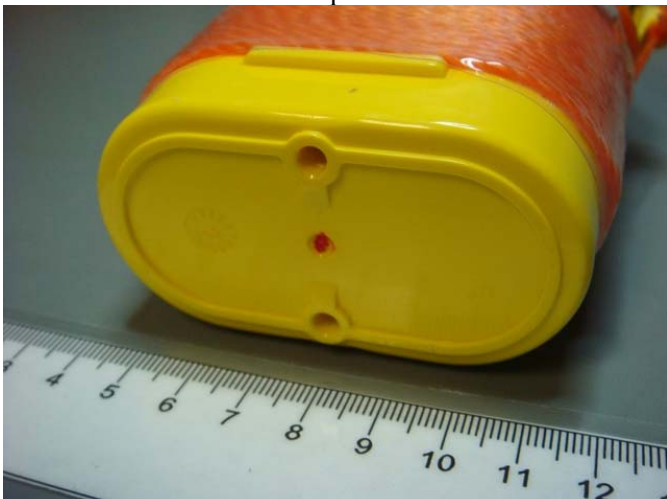
Figure 5.6 – View of the MT603G upon completion of the bump test
