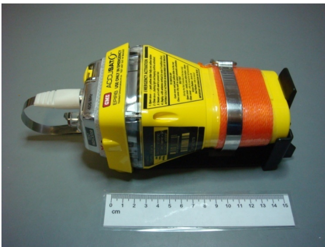
Figure 6.1 – Views of the EUT in salt fog chamber
