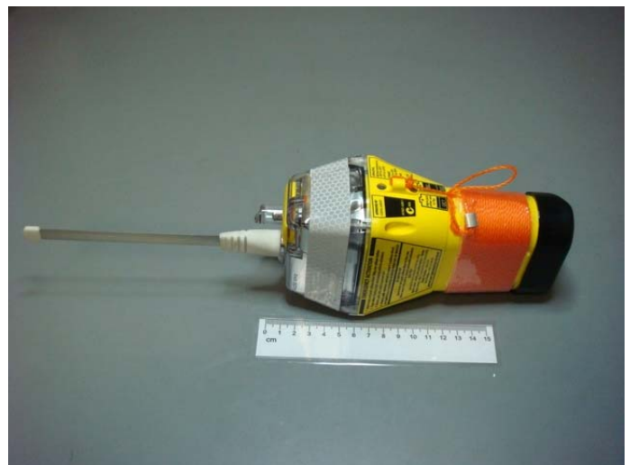
Figure 5.5 – View of the MT603FG upon completion of the bump test
