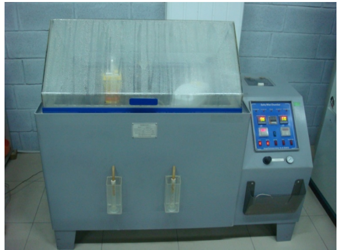
Figure 6.1 – Views of the EUT in salt fog chamber
