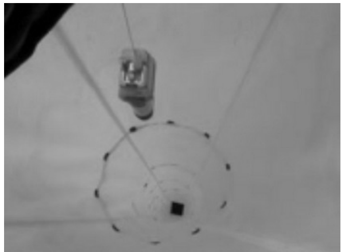
Figure 8.7 – View MT603FG dropping in water with antenna vertical up
