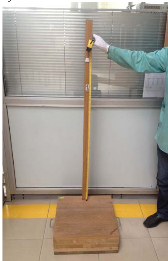
Figure 7.1 - Set-up for drop test
