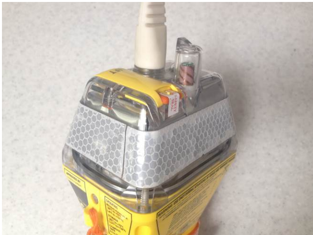
Figure 7.8 - View EUT upon completion of the drop test No indication of damage was detected at the end of test.
