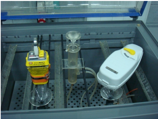
Figure 6.1 – Views of the EUT in salt fog chamber
