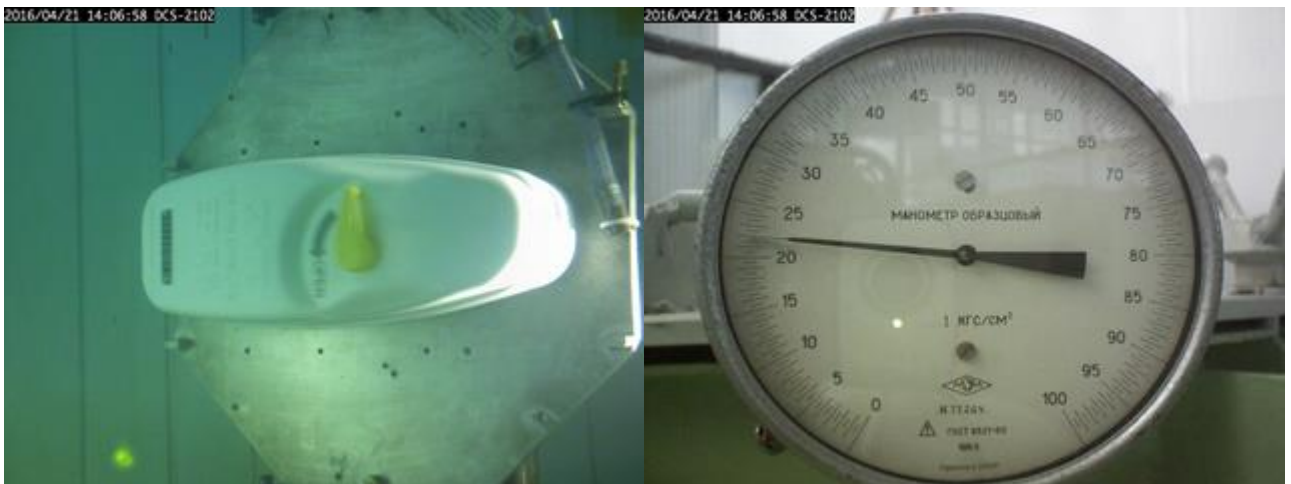
Figure 30.5 - The satellite EPIRB automatically released at Rolling 90° port orientation
