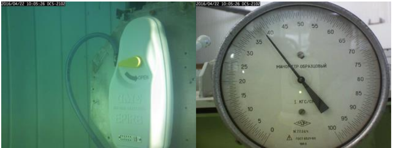
Figure 30.1 – The satellite EPIRB automatically released at normal orientation after maintained at minimum storage temperature
