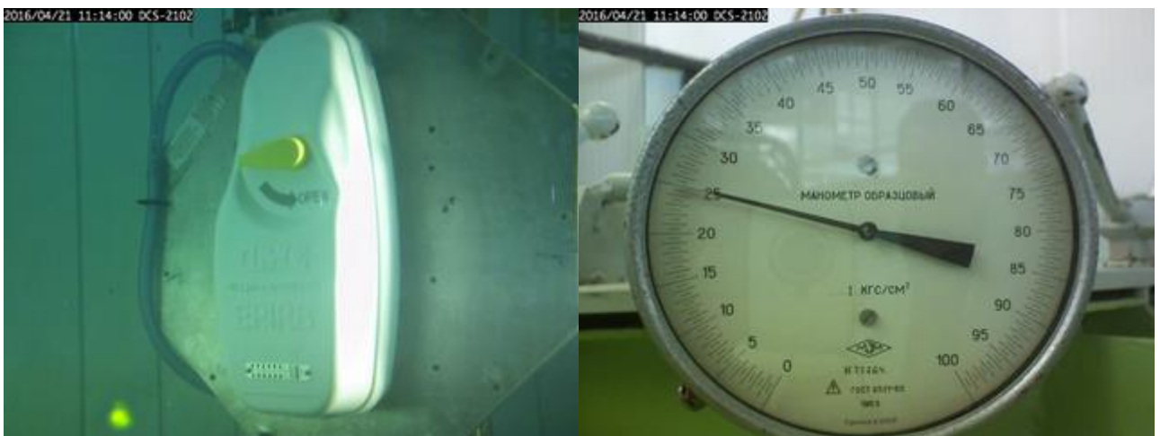
Figure 30.3 - The satellite EPIRB automatically released at normal orientation at ambient temperature
