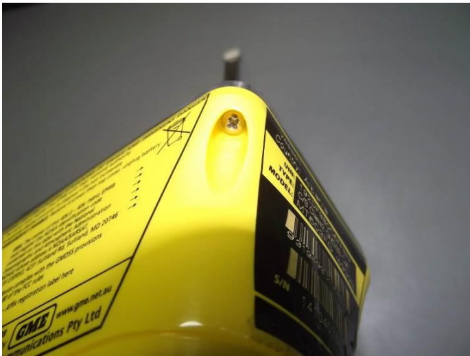
Figure 28.2 — Positions of 4 top screws
