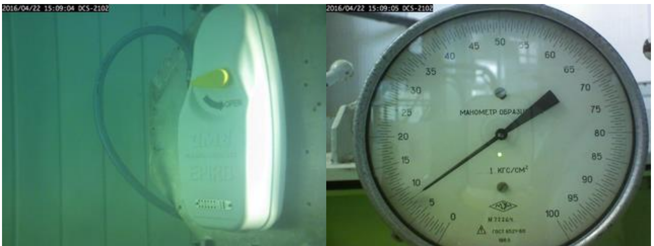
Figure 30.2 - The satellite EPIRB automatically released at normal orientation after maintained at maximum storage temperature
