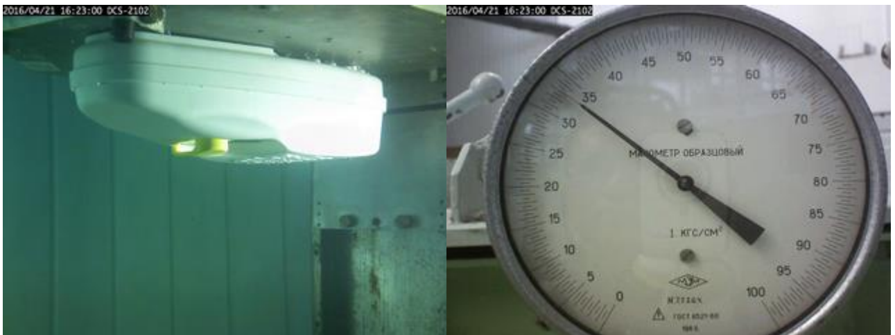
Figure 30.6 - The satellite EPIRB automatically released at Pitching 90° bow down orientation
