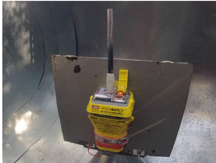
Figure 19.7 - View of EUT (MT603G) upon completion of inadvertent activation test
