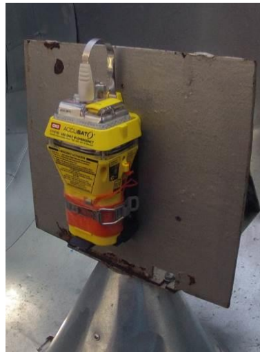
Figure 19.1 – EUT (MT603G) mounted on the rotatable support before test.
