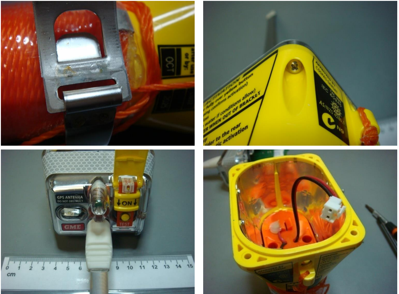
Figure 22.3 – View exterior inspection of the MT603G upon completion of the salt fog test
