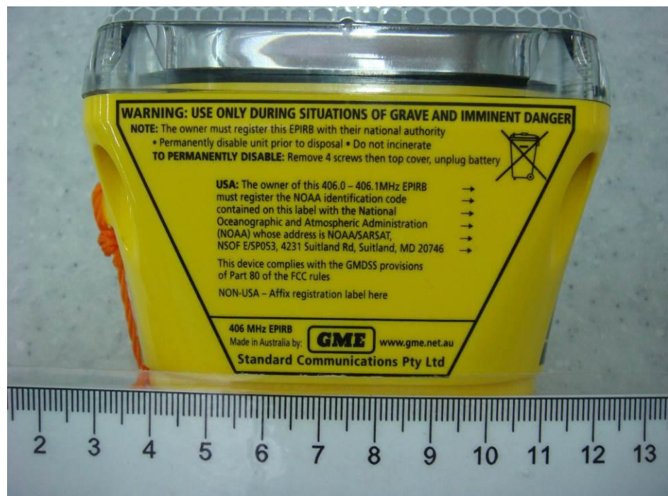
Figure 25.2 — Labelling of warning on the cover that the EPIRB is activated in emergency only
