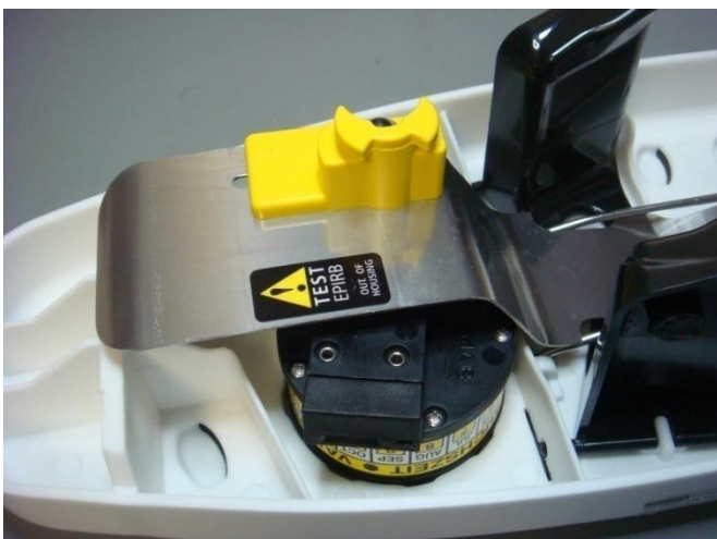
Figure 22.4 – View exterior inspection of the MT603FG upon completion of the salt fog test
