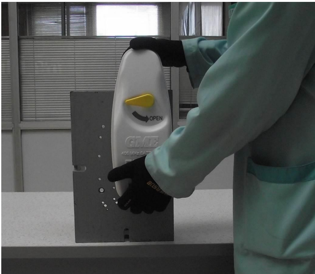
Figure 23.2 — Removing the MT603FG from Manual Release Housing (MRH)
