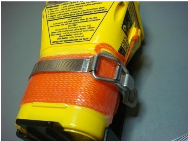
Figure 22.2 – View exterior inspection of the MT603G upon completion of the salt fog test
