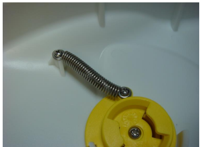
Figure 22.4 – View exterior inspection of the MT603FG upon completion of the salt fog test
