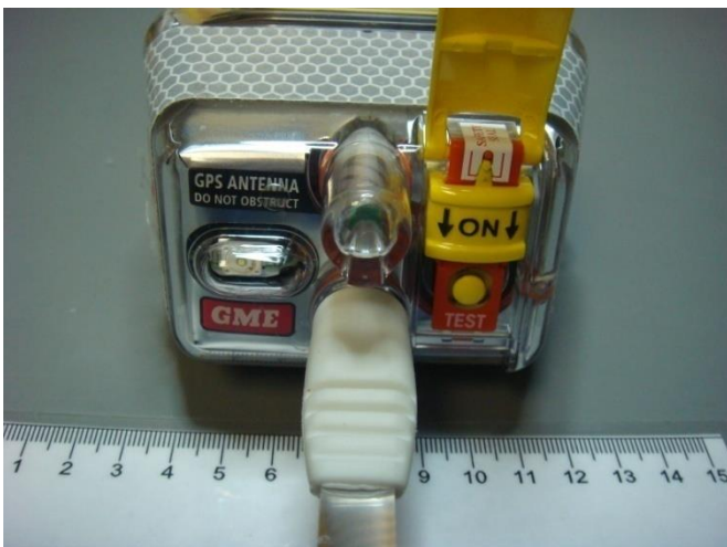
Figure 22.5 – View exterior inspection of the MT603FG upon completion of the salt fog test
