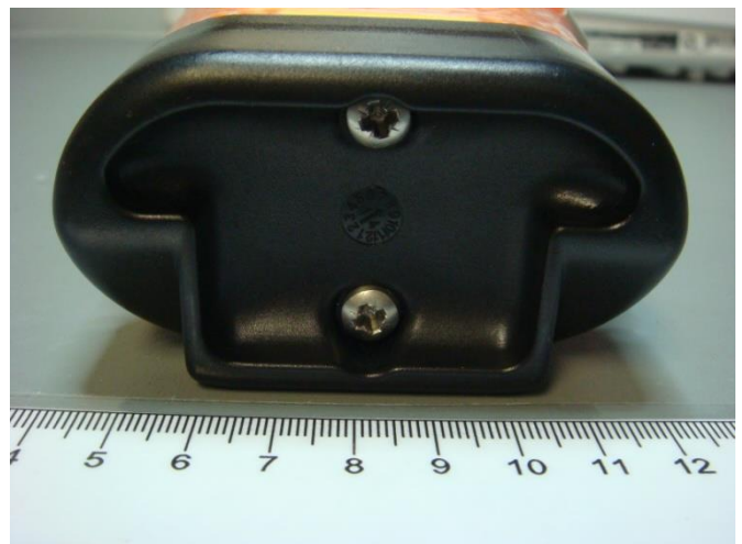
Figure 22.5 – View exterior inspection of the MT603FG upon completion of the salt fog test
