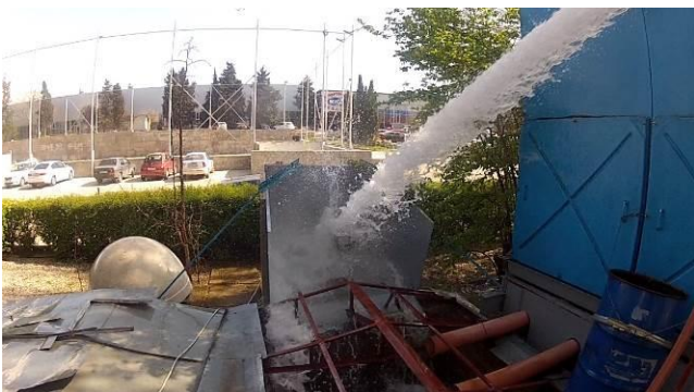
Figure 19.6 - The water strikes EUT (MT603FG) in an arc of 180°.
