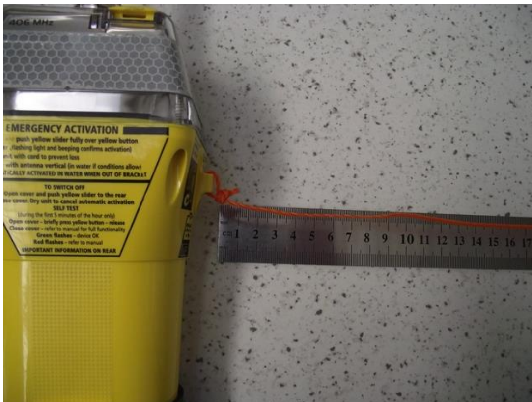
Figure 17.2 - Attaching of the lanyard
