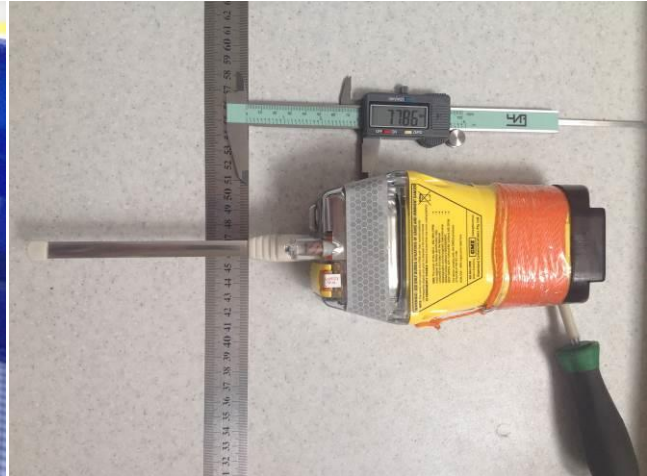
Figure 18.2 – Measuring of distance from water level to the base of antenna while EUT floating in calm fresh water
