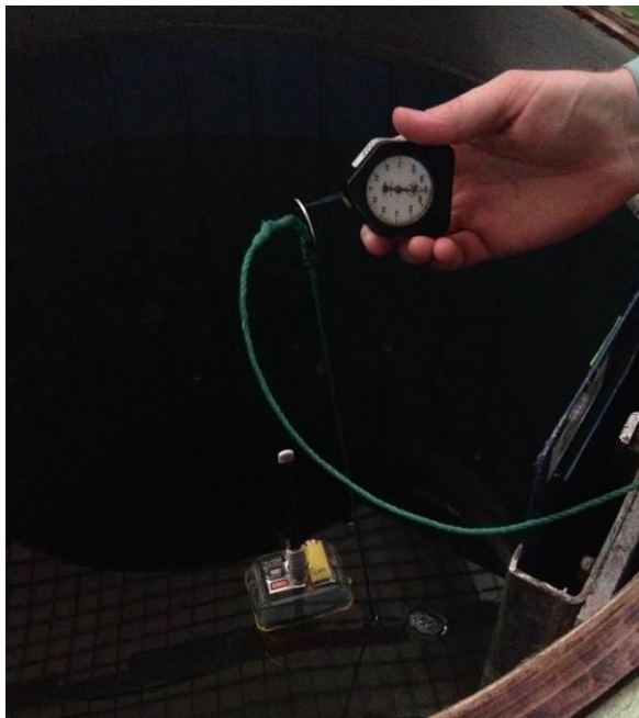
Figure 18.3 – Measuring of buoyant force
