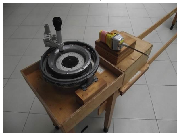
Figure 21.5 - The safety distance from EUT in operation mode to standard compass is 0.125 m (position D)
