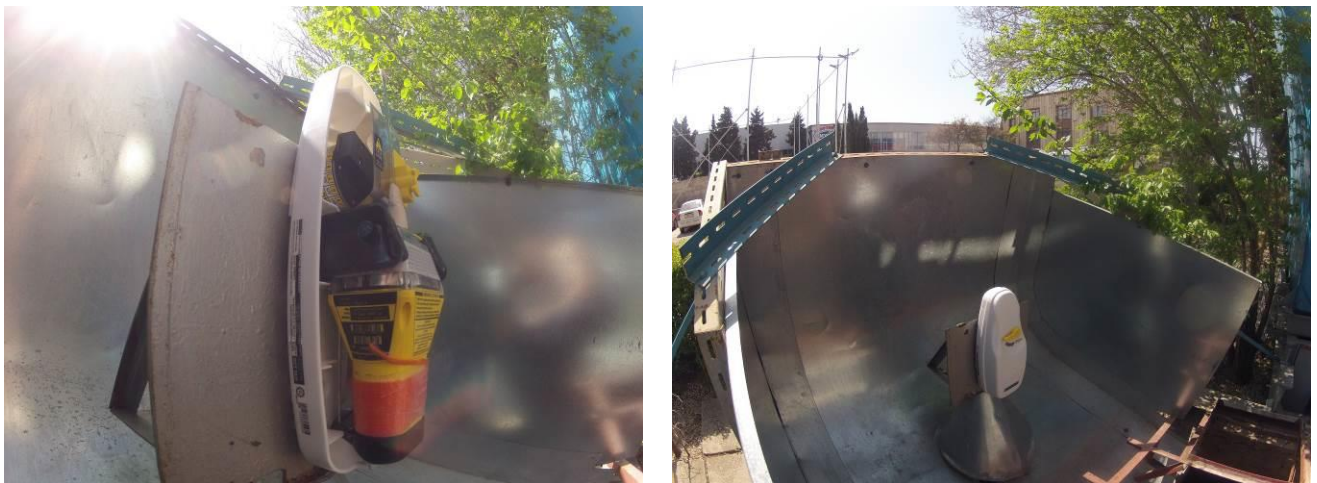
Figure 19.2 – EUT (MT603FG) mounted on the rotatable support before test.
