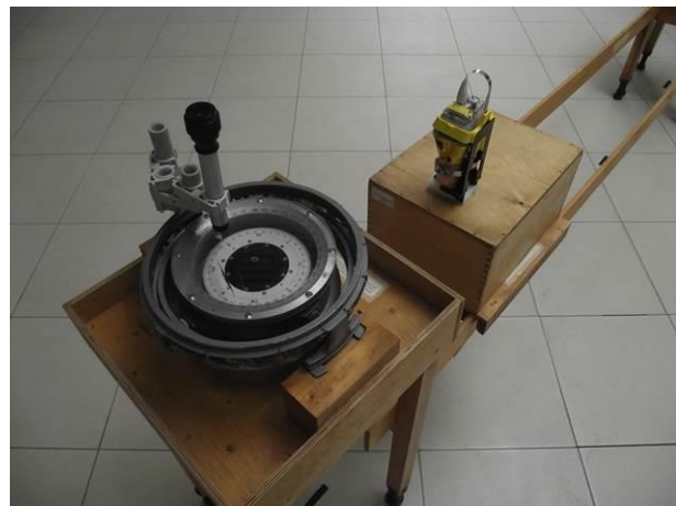
Figure 21.3 - The safety distance from EUT in stand-by mode to standard compass is 0.28 m (position F)
