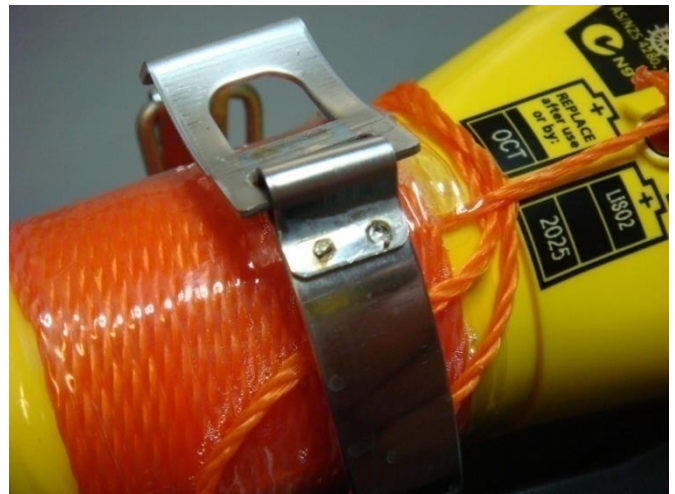
Figure 22.2 – View exterior inspection of the MT603G upon completion of the salt fog test
