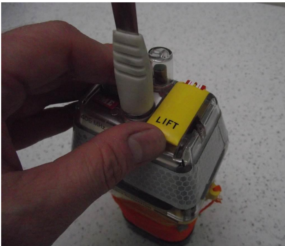
Figure 24.1 - Activator of distress signal
