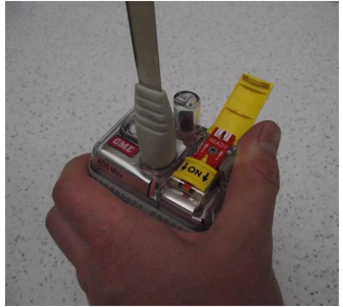
Figure 24.4 - Manual distress alert initiation step 3
