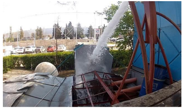
Figure 19.5 - The water strikes EUT (MT603G) in an arc of 180°.
