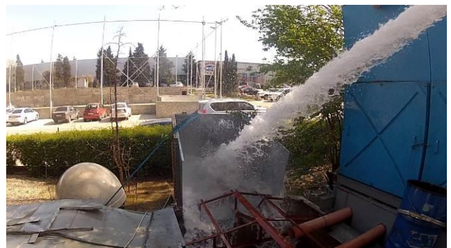
Figure 19.6 - The water strikes EUT (MT603FG) in an arc of 180°.
