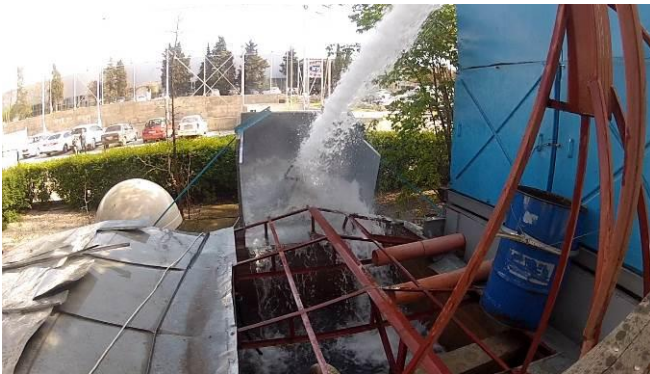
Figure 19.5 - The water strikes EUT (MT603G) in an arc of 180°.
