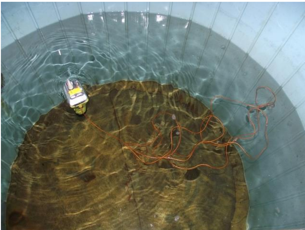
Figure 17.4 – Checking buoyancy of the lanyard
