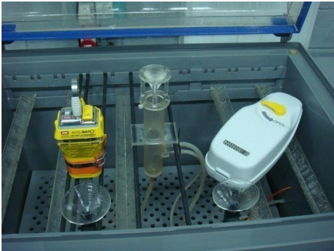
Figure 22.1 – Views of the EUT in salt fog chamber
