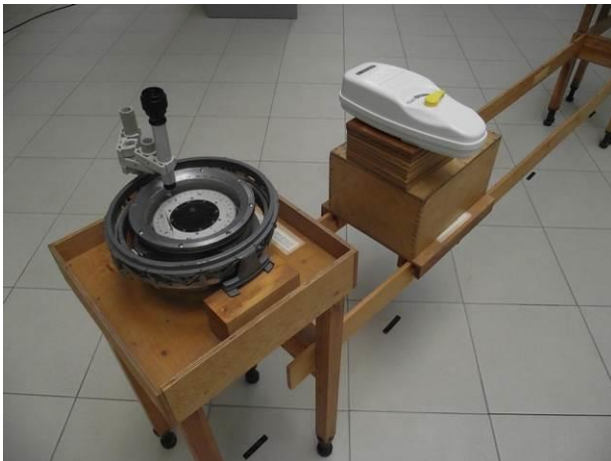
Figure 21.7 - The safety distance from EUT to standard compass is 0.74 m (position E).
