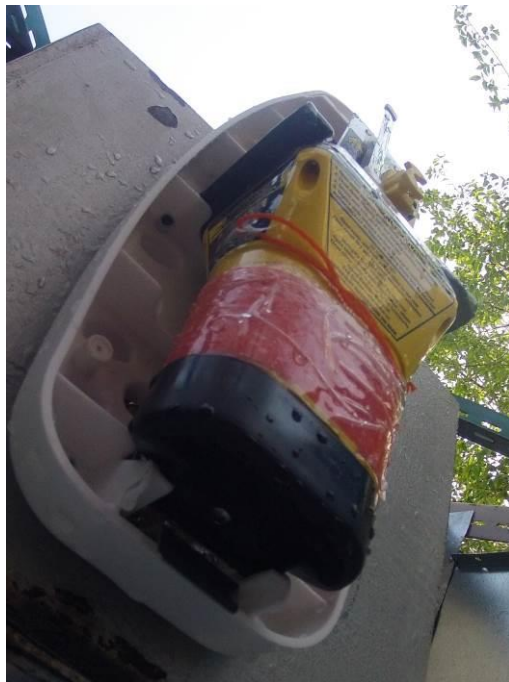
Figure 19.8 - View of EUT (MT603FG) upon completion of inadvertent activation test
