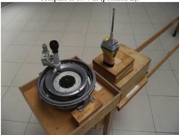
Figure 21.9 - The safety distance from EUT in operation mode to standard compass is 0.23 m (position B)
