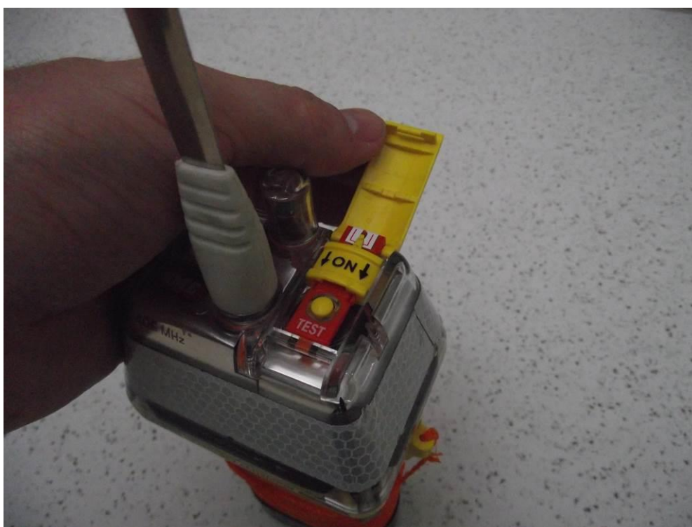
Figure 24.2 - Manual distress alert initiation step 1
