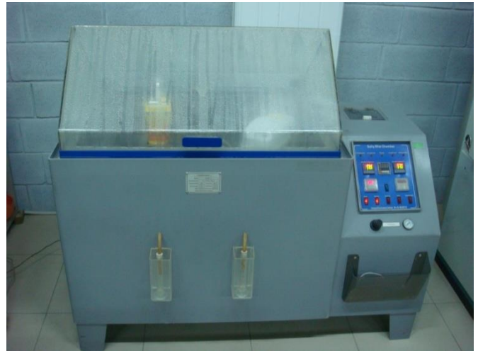
Figure 22.1 – Views of the EUT in salt fog chamber
