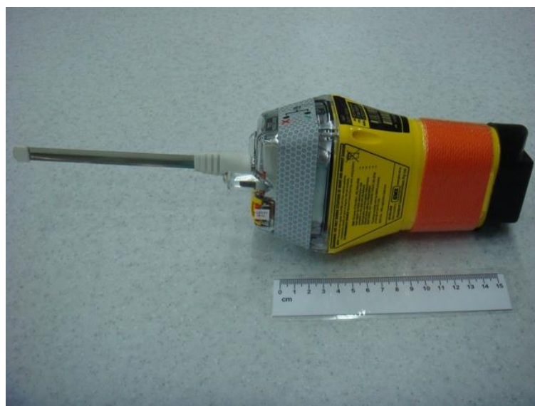
Figure 28.1- EPIRB is a single integral unit
