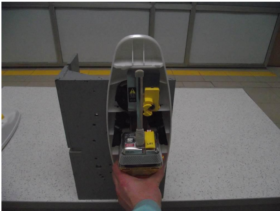
Figure 24.5 - Removed EUT from the Manual Release Housing (MRH) and Manual bracket. EPIRB was not automatically activated
