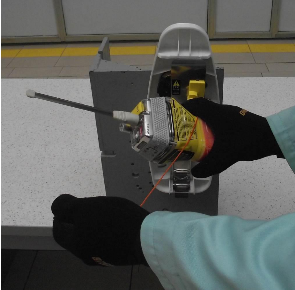
Figure 23.11 — Deployment of the lanyard
