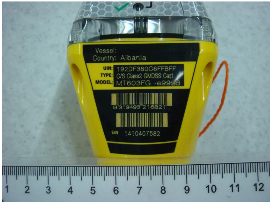
Figure 25.5— Labelling of vessel (Vessel Name) and identifier number (UIN)
