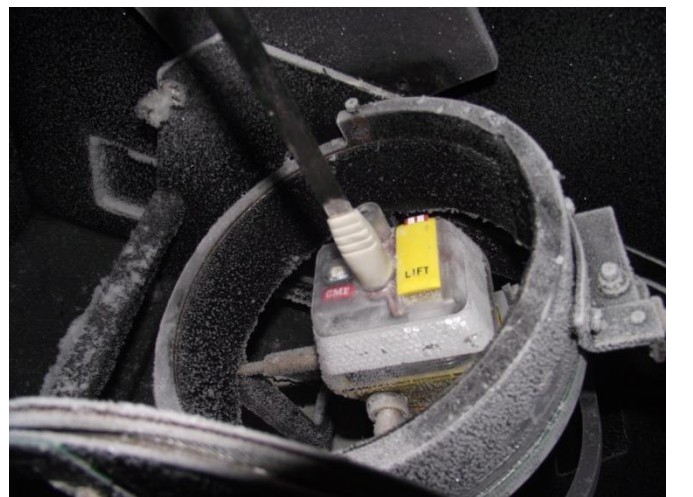
Figure 15.7 –View of the EUT upon completion of the low-duty cycle test at minimum temperature
