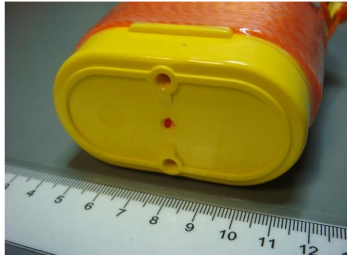
Figure 5.7 – View of the MT603G upon completion of the ruggedness test
