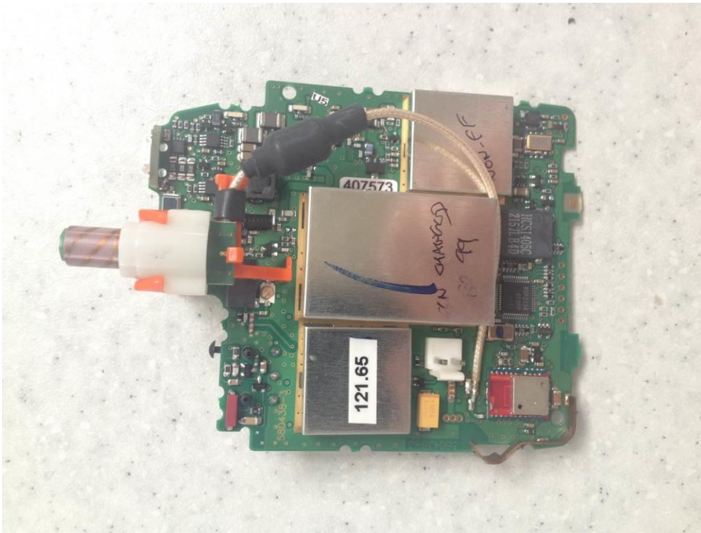
Figure 8.5 – View of the interiors of the Beacon upon completion of the Thermal Shock Test and Immersion Test
