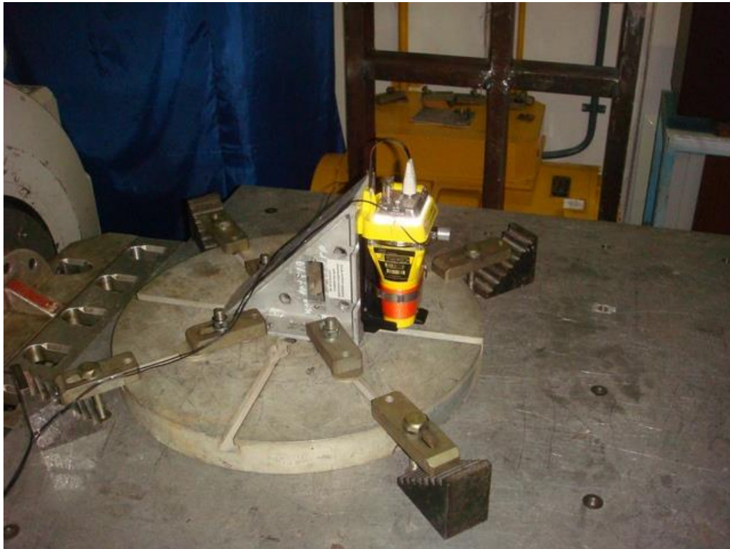
Figure 4.3- General view of the horizontal axis X vibration test (MT603G)
