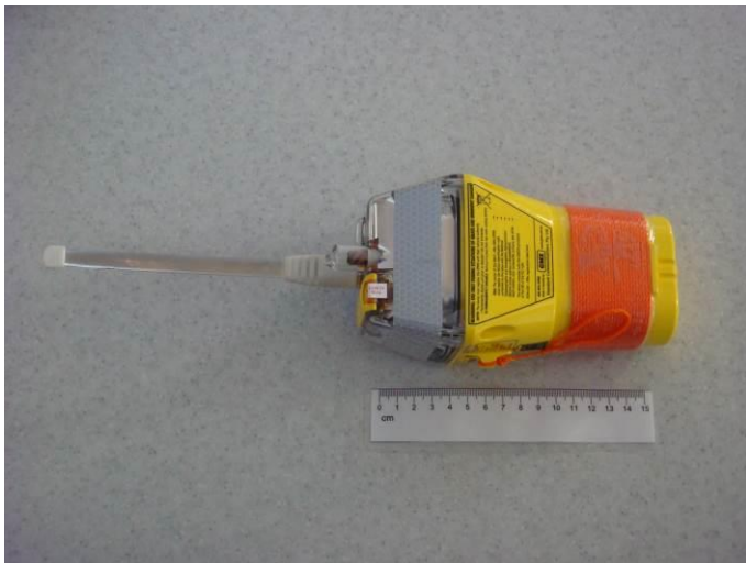
Figure 5.4 – View of the MT603G upon completion of the ruggedness test
