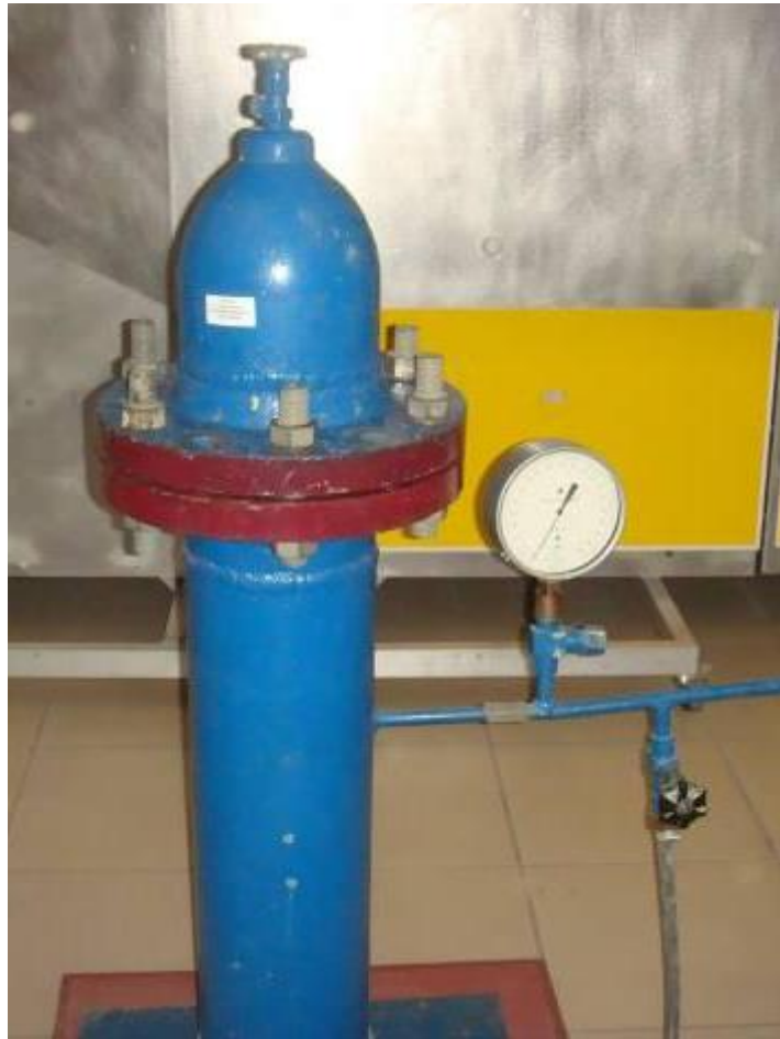
Figure 8.3 — Hydraulic pressure set-up (1 bar)
