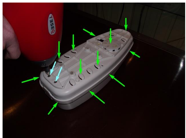
Figure 12.2 - Site for Test of Immunity to Electrostatic Discharge
