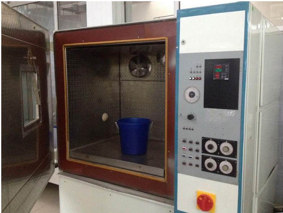
Figure 8.1 – View of the Beacon in the temperature test chamber during the Thermal Shock Test
