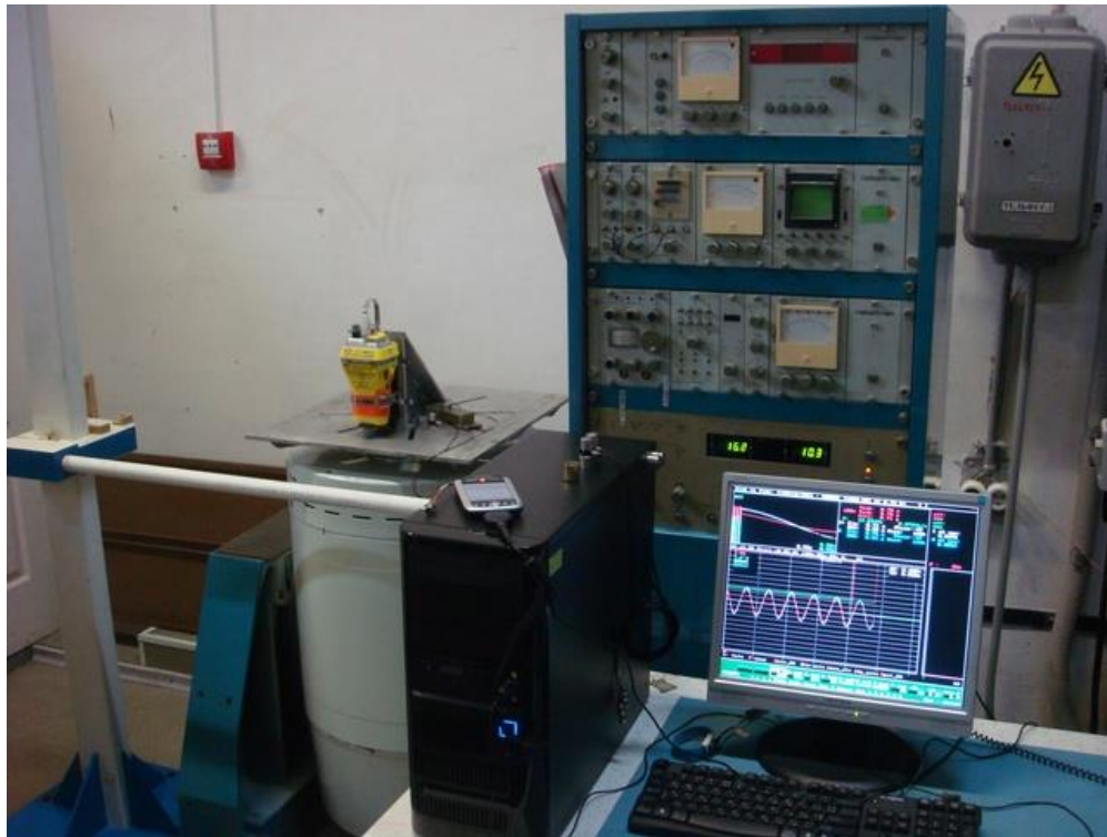
Figure 4.1 - General view of the test site vertical vibration (MT603G)
