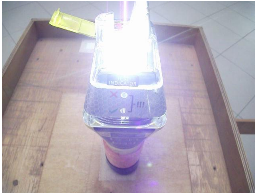
Figure 13.4 — The strobe LED is flashes.
