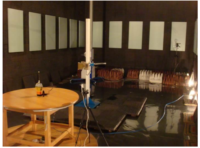
Figure 11.3 - General view of immunity test set-up. Vertical polarization.
