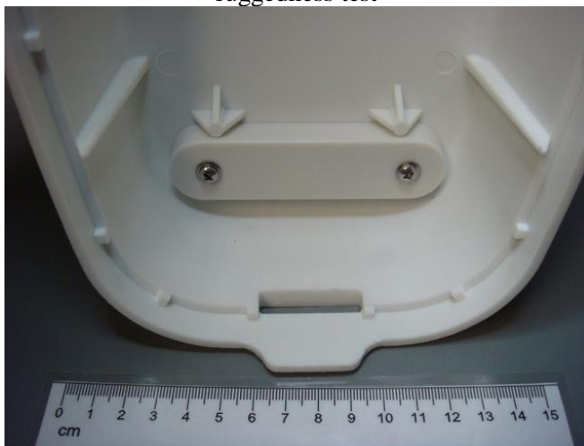
Figure 5.8– View of the MRH(MT603FG) upon completion of the ruggedness test
