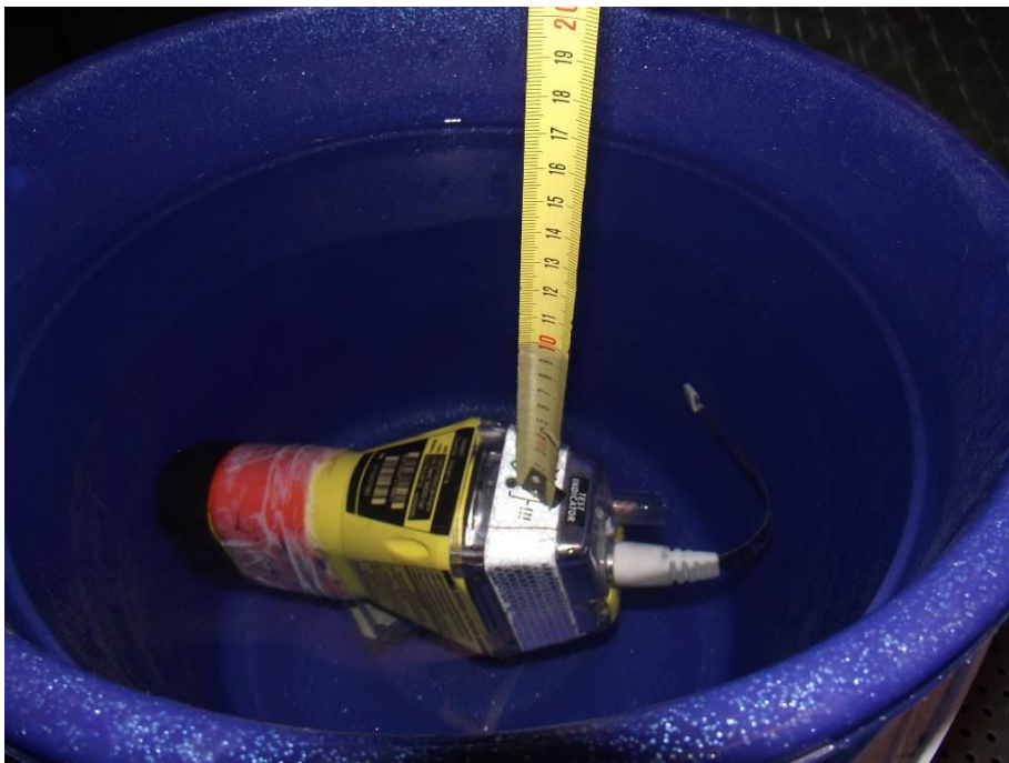
Figure 8.2 —View of the Beacon in the water during the Thermal Shock Test
