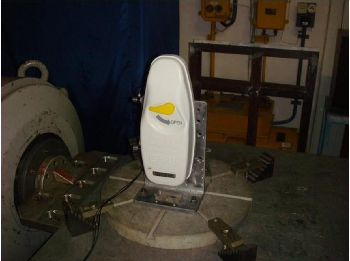
Figure 4.12 - General view of the horizontal Y vibration test (MT603FG)
