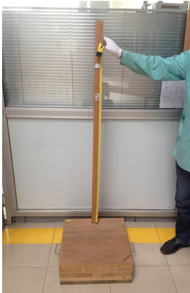
Figure 6.1 - Set-up for drop test
