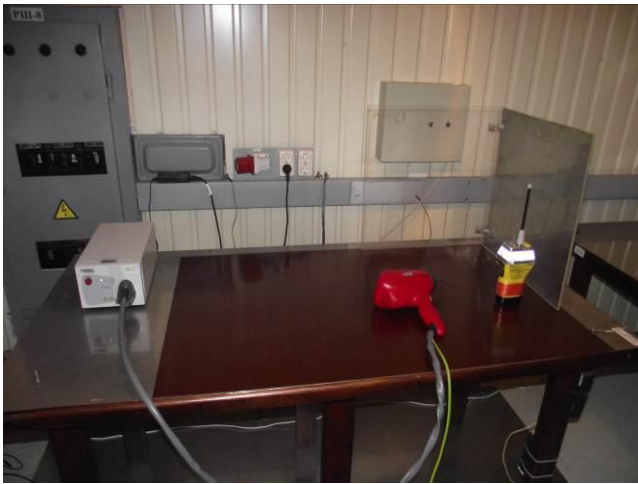
Figure 12.2 - Site for Test of Immunity to Electrostatic Discharge
