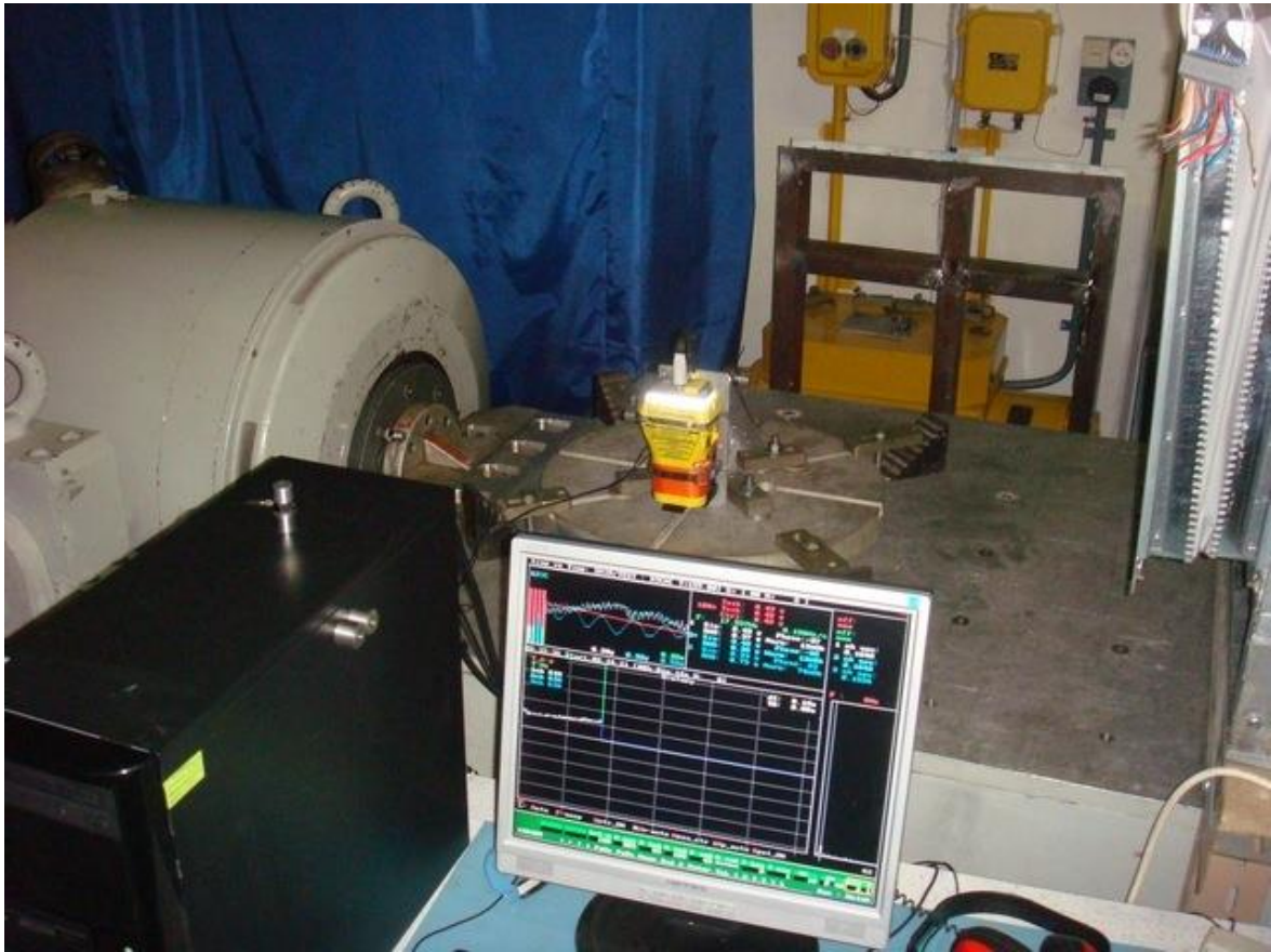
Figure 4.5 - General view of the horizontal Y vibration test (MT603G)
