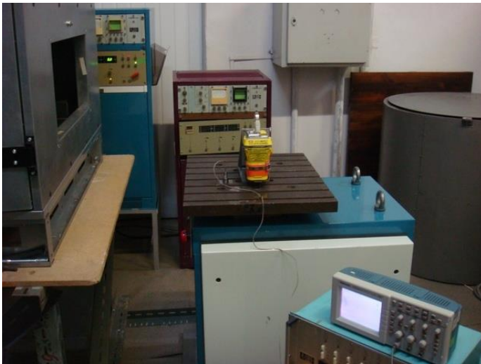
Figure 5.2 - Test Set-up. Vertical axis of the MT603G
