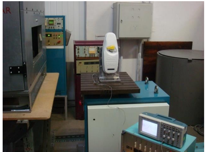
Figure 5.3 - Test Set-up. Vertical axis of the MT603FG
