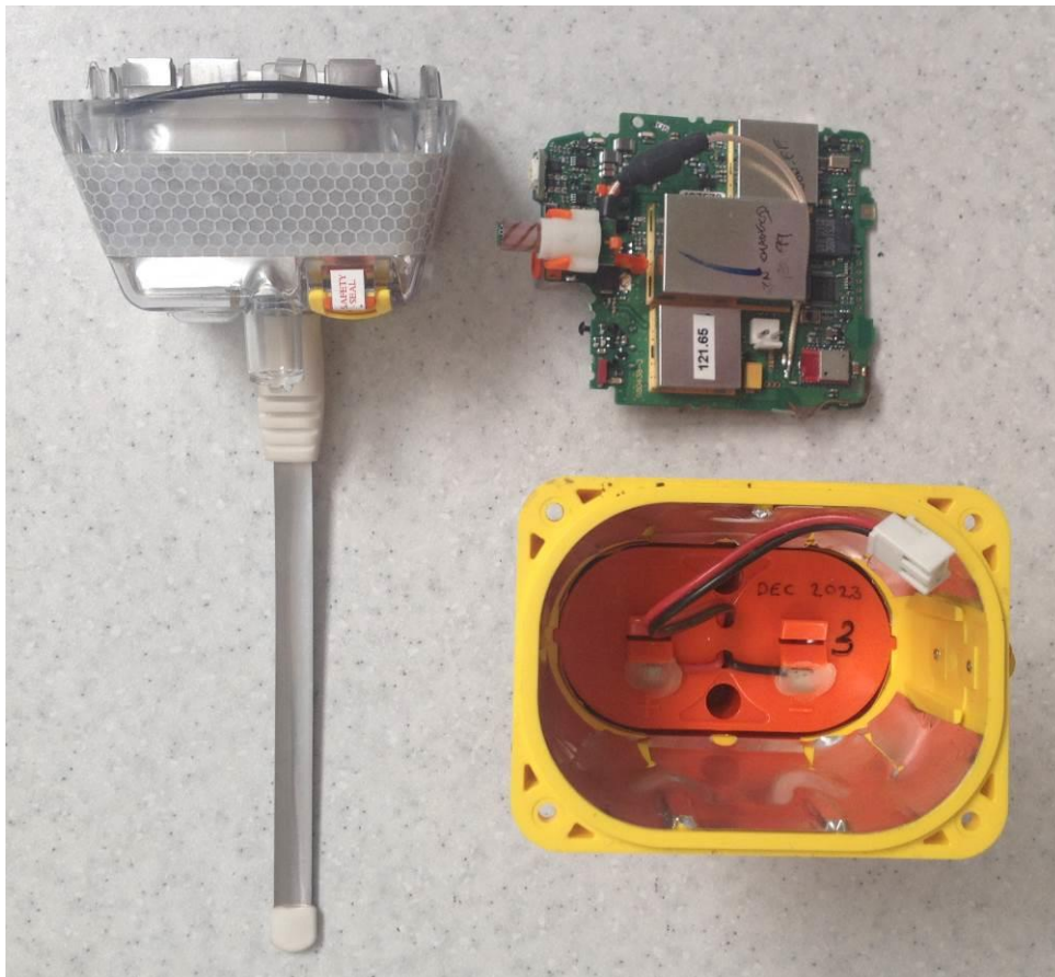
Figure 8.4 – View of the interiors of the Beacon upon completion of the Thermal Shock Test and Immersion Test
