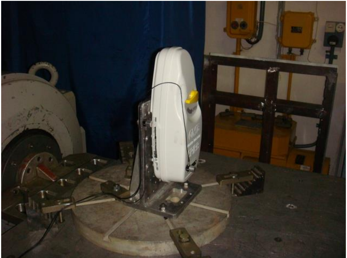
Figure 4.10- General view of the horizontal axis X vibration test (MT603FG)
