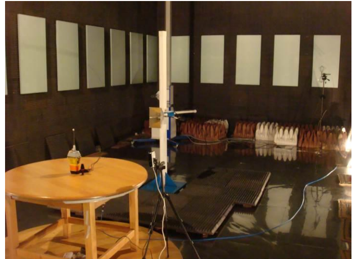
Figure 11.4 - General view of immunity test set-up. Horizontal polarization.
