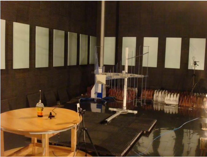
Figure 11.3 - General view of immunity test set-up. Vertical polarization.
