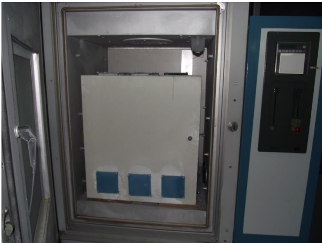
Figure 15.4 –General view of rotation and inclination device inside of the climatic chamber
