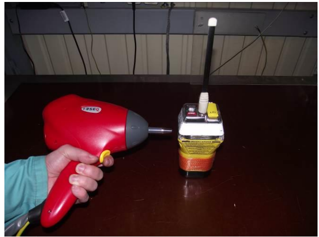
Figure 12.2 - Site for Test of Immunity to Electrostatic Discharge
