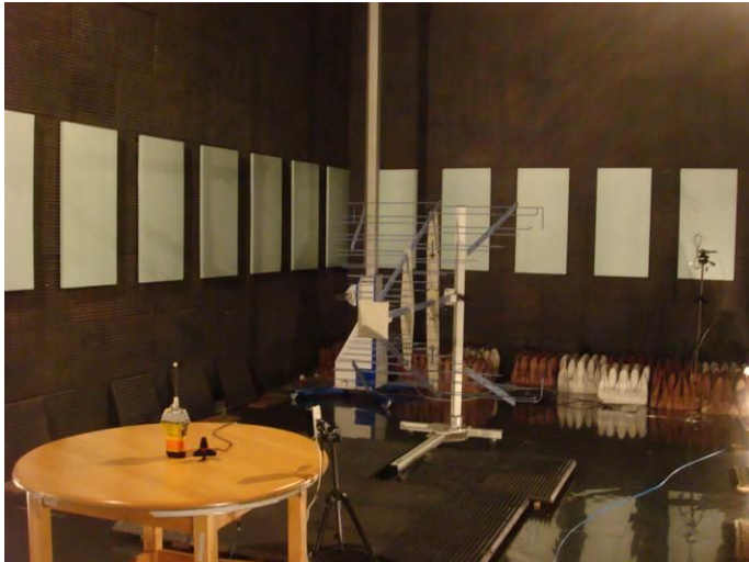
Figure 11.4 - General view of immunity test set-up. Horizontal polarization.
