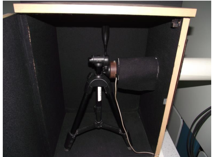
Figure 15.3 –General view of graphic luxmeter
