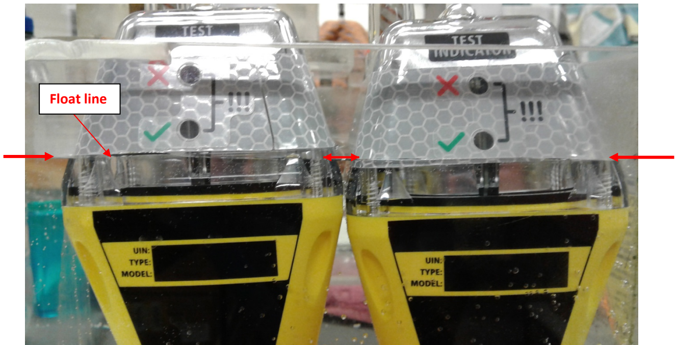
Figure 1 MT603G (left) and MT603FG (right) side-by-side in a water tank – zoomed in
