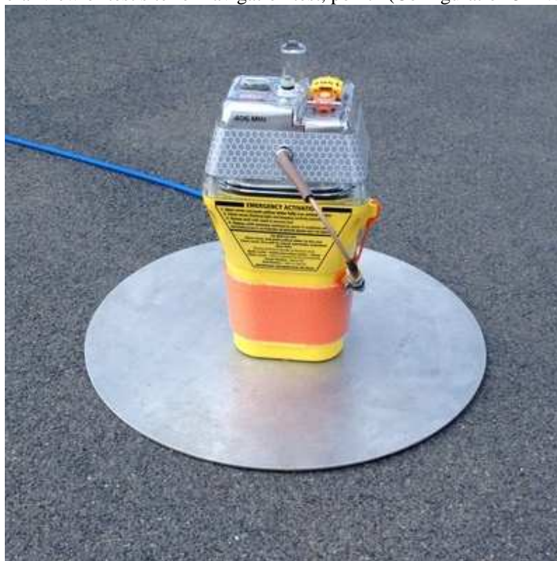
Fig. 5.10.2 — General view of test site for navigation test, point 1 (Configuration 7 – Beacon on ground plan).
