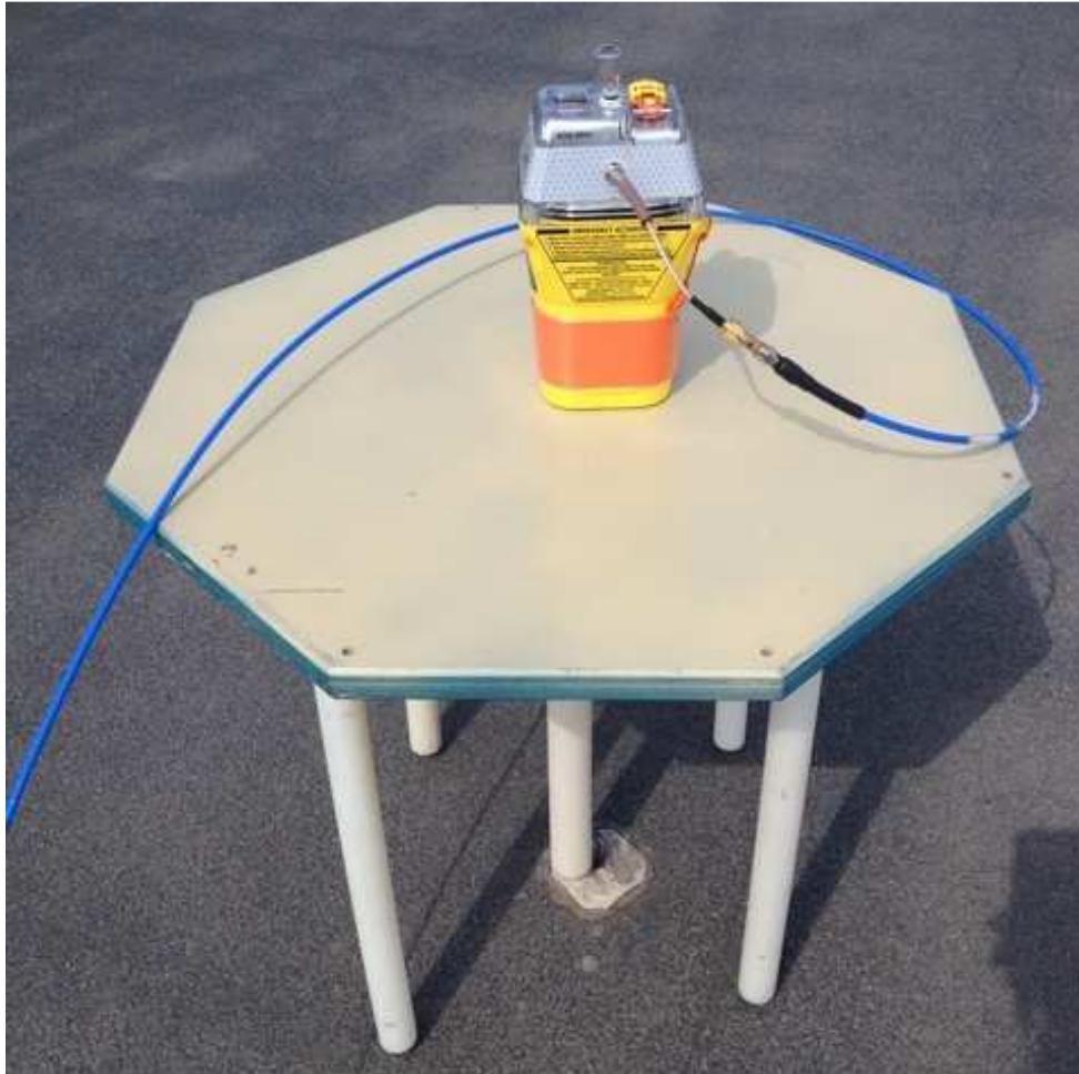
Fig. 5.10.3 — General view of test site for navigation test, point 1 (Configuration 8 - Beacon above ground plane).
