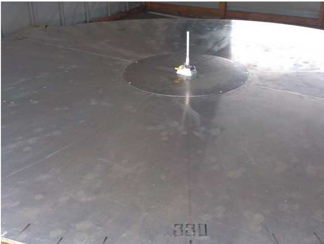
Fig 5.10.7 — General view of antenna test place at configuration 1 (section 4.5 C/S T.007) (beacon operated on «water» ground plane).
