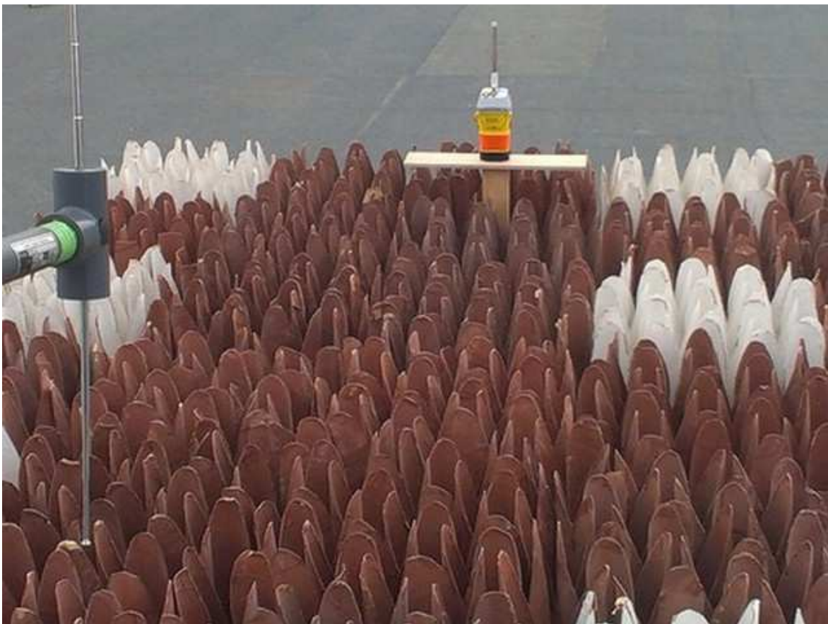
Fig 5.10.8 — General view of antenna test place at configuration 4 (section 4.5 C/S T.007) (beacon operating above ground plane).
