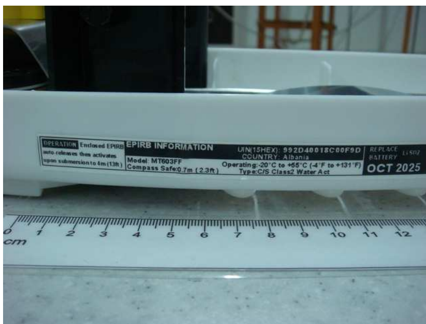
Figure 3.5 – The view of MT603FG labels on the auto-release housing (s/n 1410407582).
