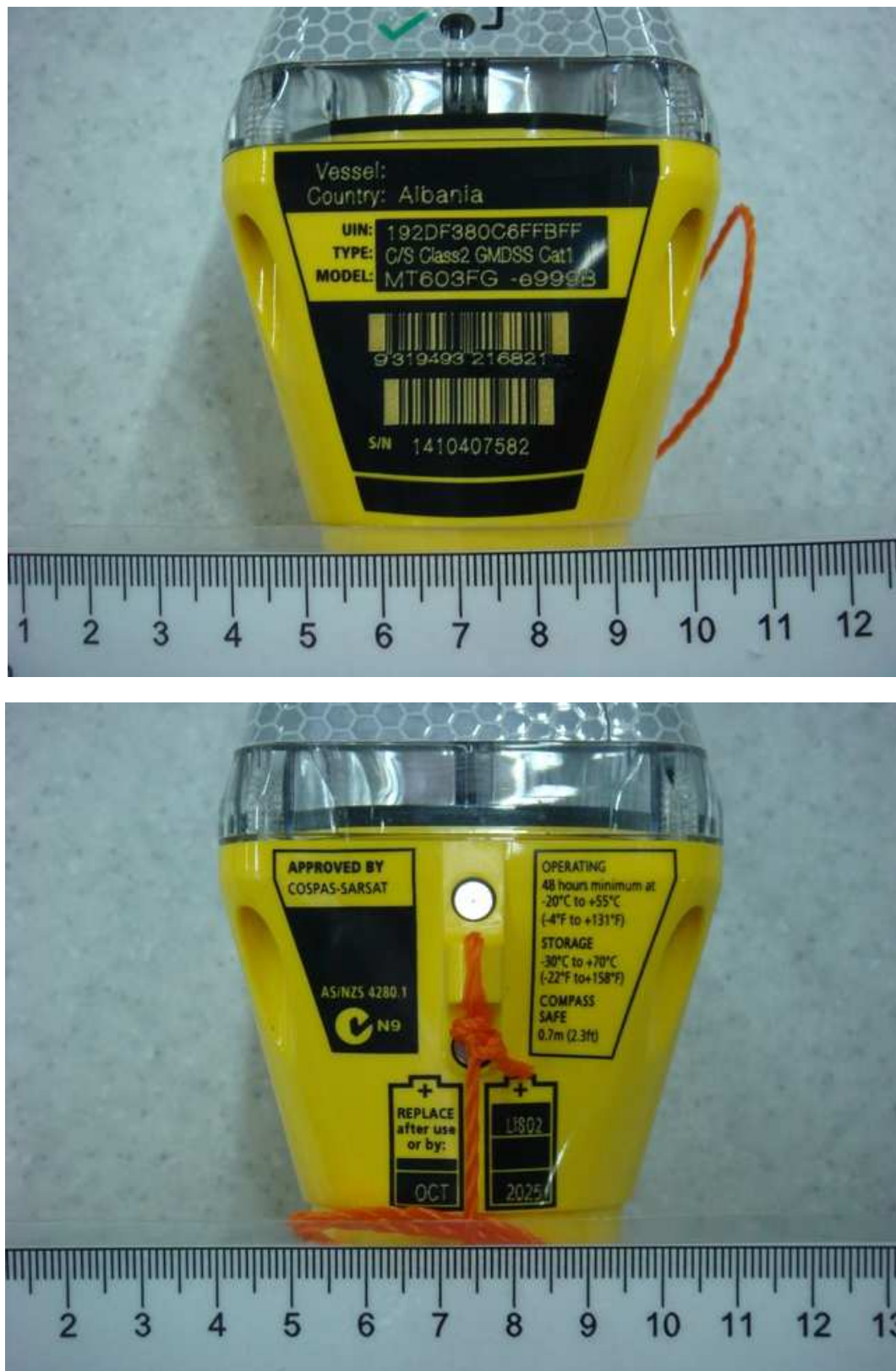
Figure 3.6 – The view of MT603FG labels (s/n 1410407582).
