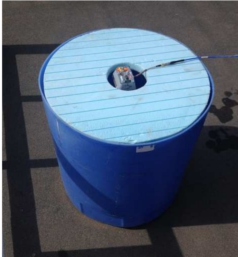
Fig. 5.10.1 — General view of test site for navigation test, point 1(Configuration 5 – Water ground plane).
