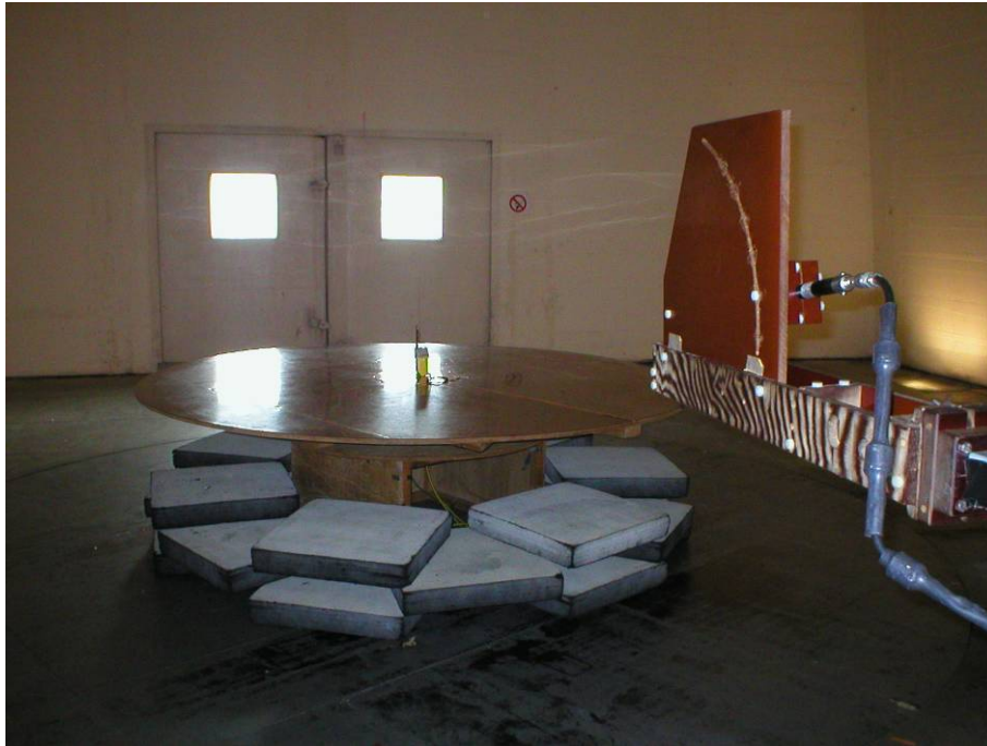
Antenna Characteristics Testing (EUT on ground plane (2.5m dia. 0.75m height) – Antenna Deployed
