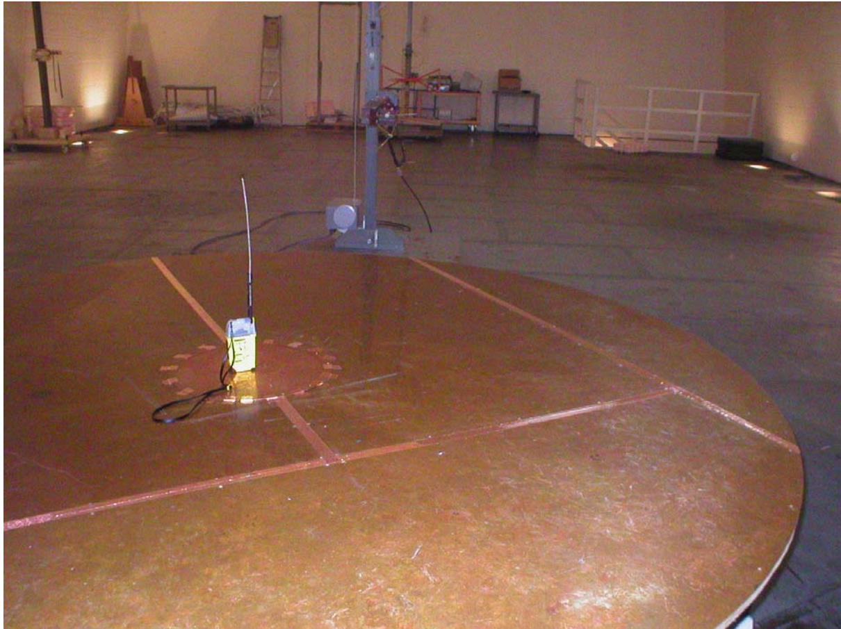
Antenna Characteristics Testing (EUT on ground plane (2.5m dia. 0.75m height) – Antenna Deployed Build State 1
