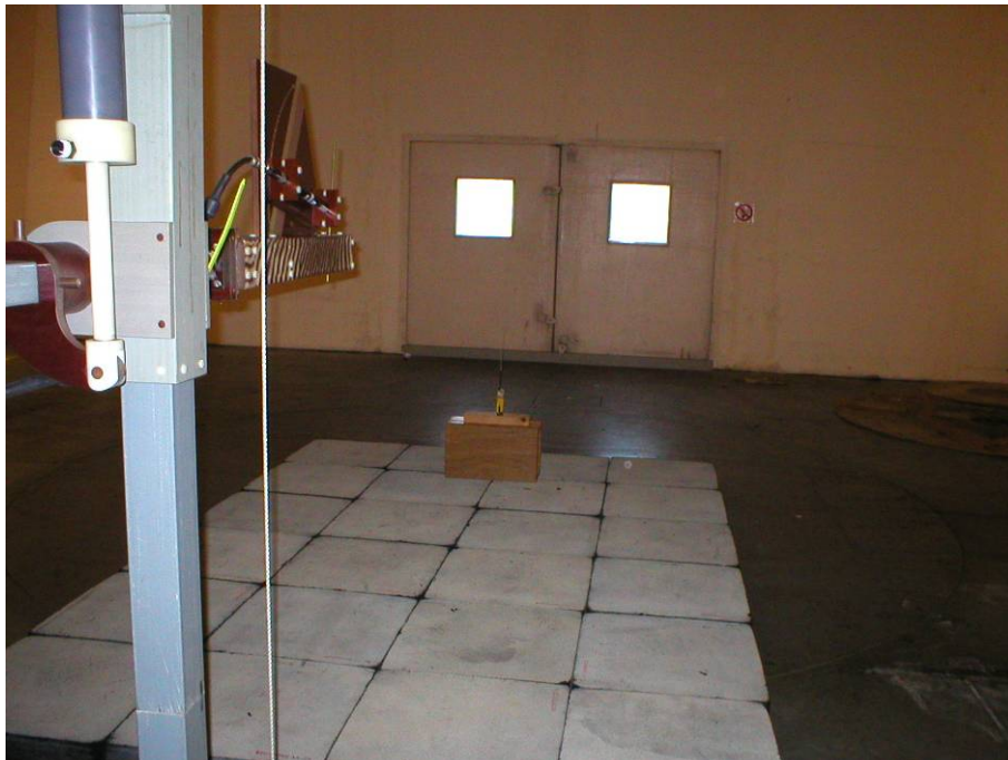
Antenna Characteristics Testing (EUT simulated above dry ground) – Antenna Deployed
