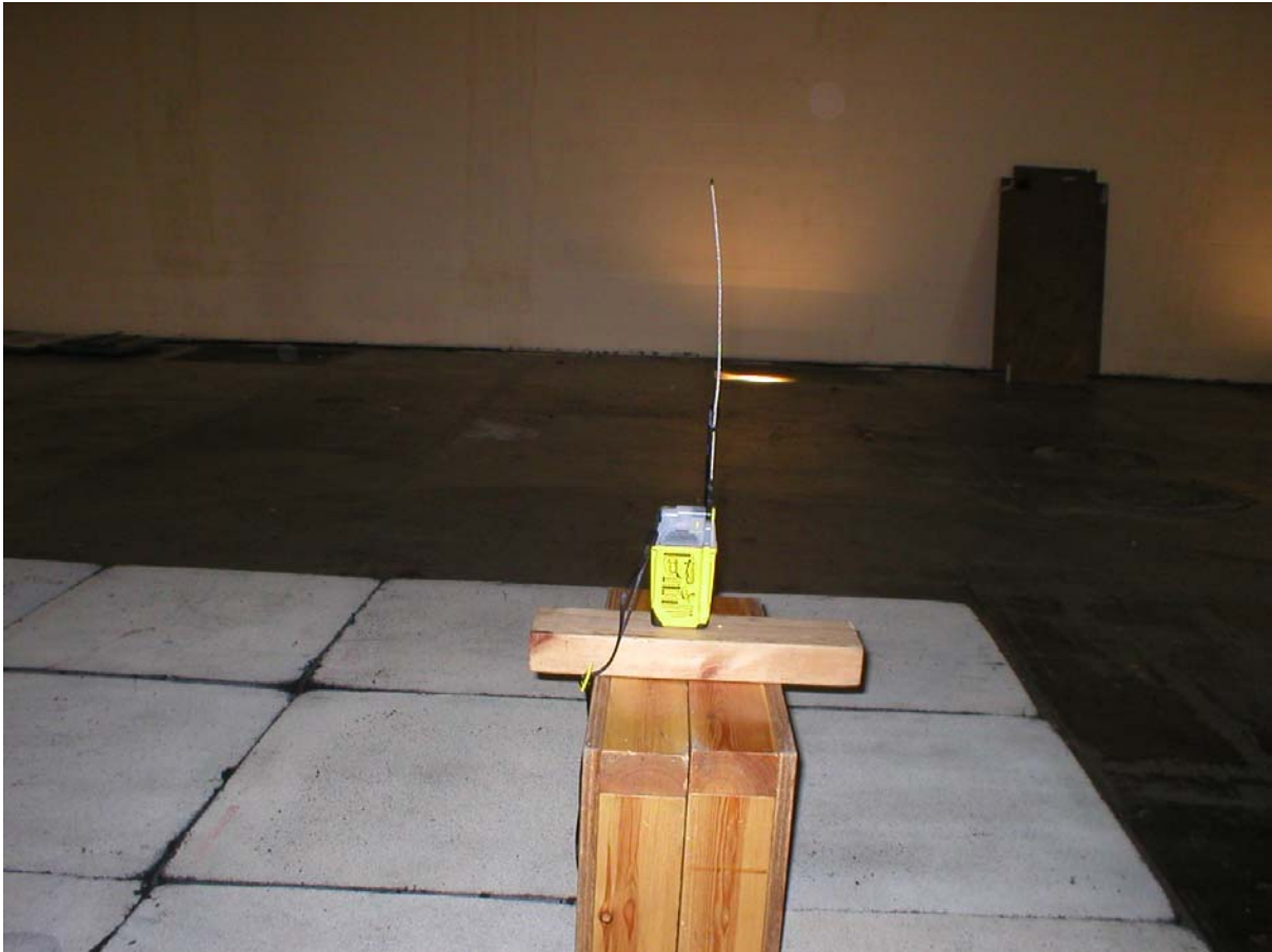
Antenna Characteristics Testing (EUT simulated above dry ground) – Antenna Deployed Build State 1
