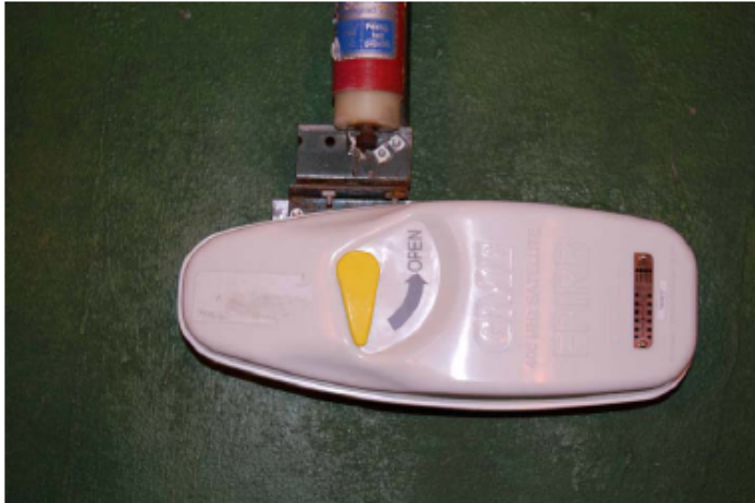
EPIRB mounted on the plunger pole ready test, Rolling 90° attitude.
