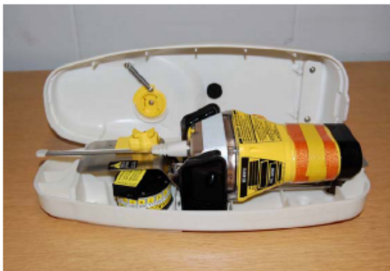
The release mechanism primed ready for the cover to be put on, Hammar H20 release can be seen to the left of centre and when hydrostatically triggered will cut through the black nylon post that holds the cover on. The sprung metal hinged release plate will then push up and away the GME beacon. Second photo shows detail of the angle piece on the clear antenna cover that was included before the test sessions started to ensure clean separation from the release plate.
