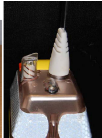
The release mechanism primed ready for the cover to be put on, Hammar H20 release can be seen to the left of centre and when hydrostatically triggered will cut through the black nylon post that holds the cover on. The sprung metal hinged release plate will then push up and away the GME beacon. Second photo shows detail of the angle piece on the clear antenna cover that was included before the test sessions started to ensure clean separation from the release plate.
