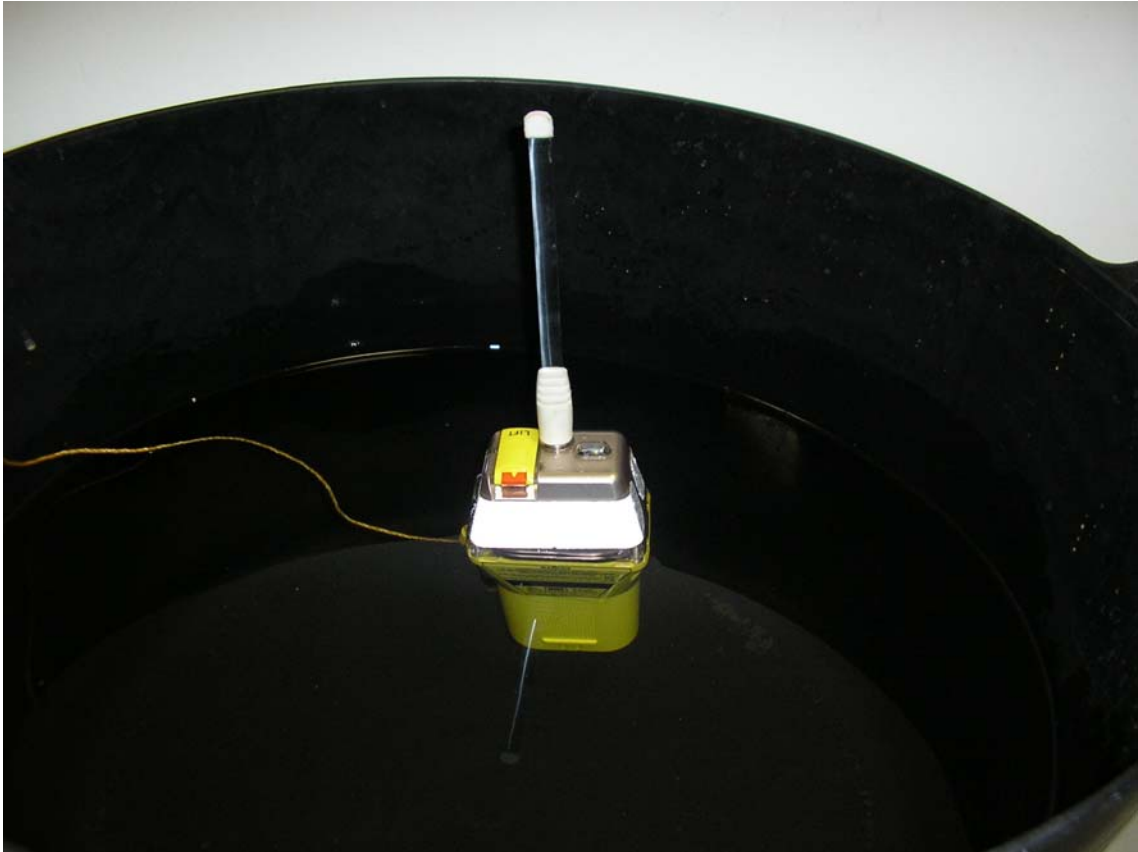
EUT Immersed In Fresh Water
