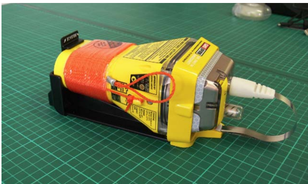
Picture 5 - MT403G in manual release bracket
