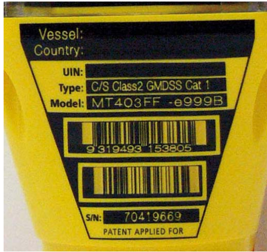
Picture 3 - Sample MT403FF laser marking detail (Example shown, to be programmed by distributor)
