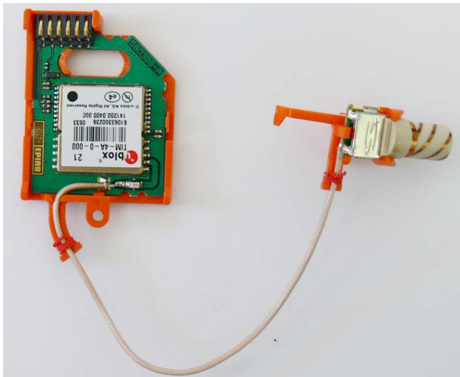
Picture 3 - GPS Application Module assembly (MT403G and MT403FG only)
