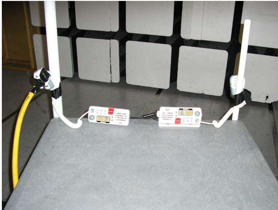
Photograph of Radiated Emissions Test Setup
