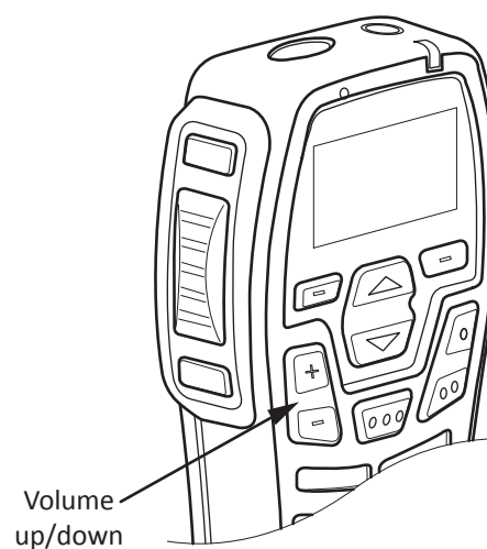
Figure 8 - Turning radio volume up and down on controller microphone
