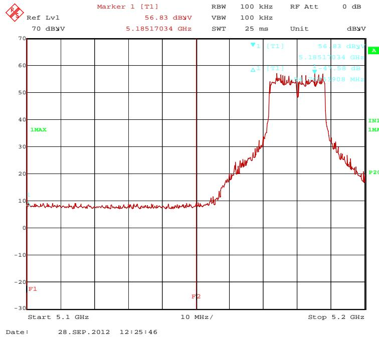
123441\_42.wmf: Radiated band-edge compliance (transmitting at channel 48 in a-mode):
