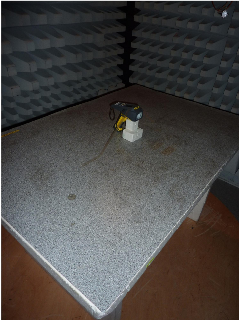
123441_1.JPG: Test setup fully anechoic chamber
