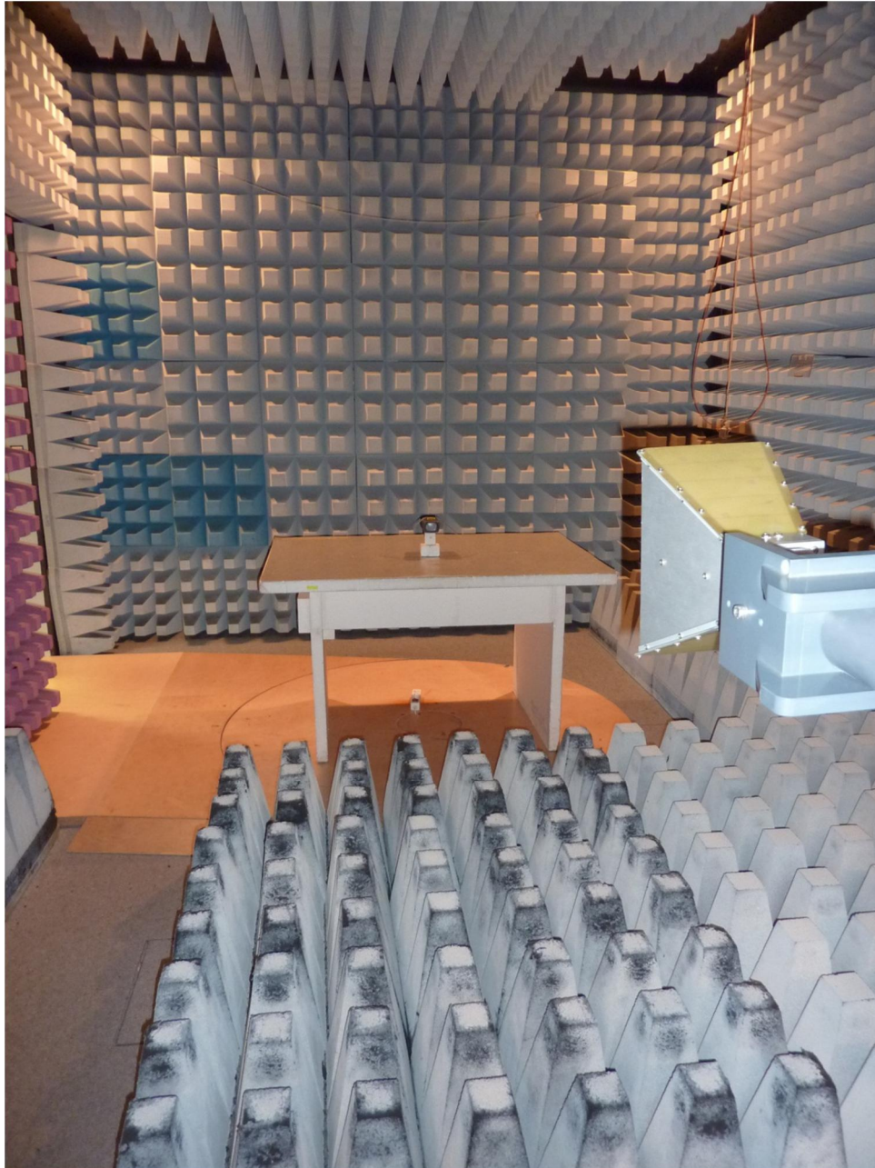
123441_2.JPG: Test setup fully anechoic chamber
