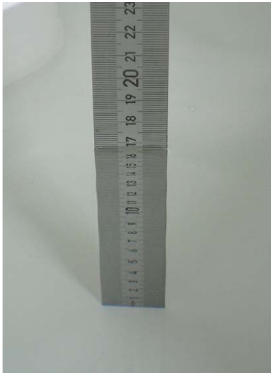
Fig. 18: Liquid depth for IEEE 802.11 b/g Body measurements
