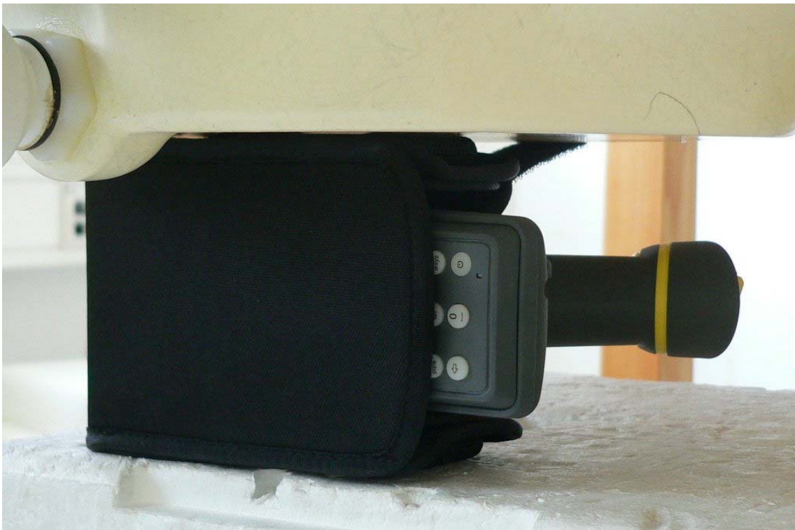
Fig. 17: Body worn configuration, position 2 with holster, right edge of display in direct contact against the flat phantom.
