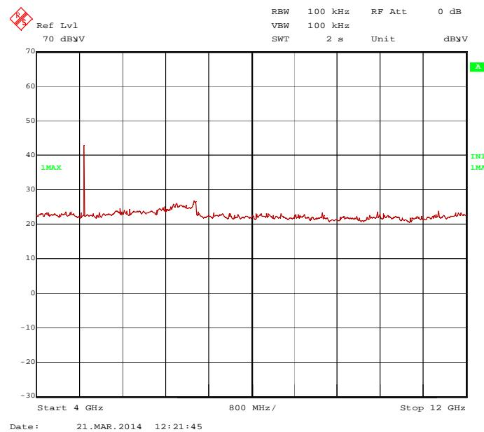
140269\_12-18GHz\_2441.wmf: Spurious emissions from 12 GHz to 18 GHz:
