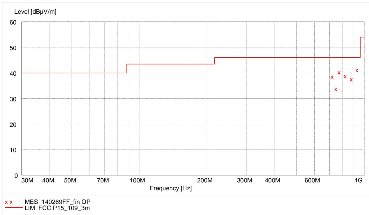
The results of the standard subsequent measurement on the open area test site are indicated in the table below. The limits as well as the measured results (levels) refer to the above mentioned standard while taking account of the specified requirements for a 3 m measuring distance.
