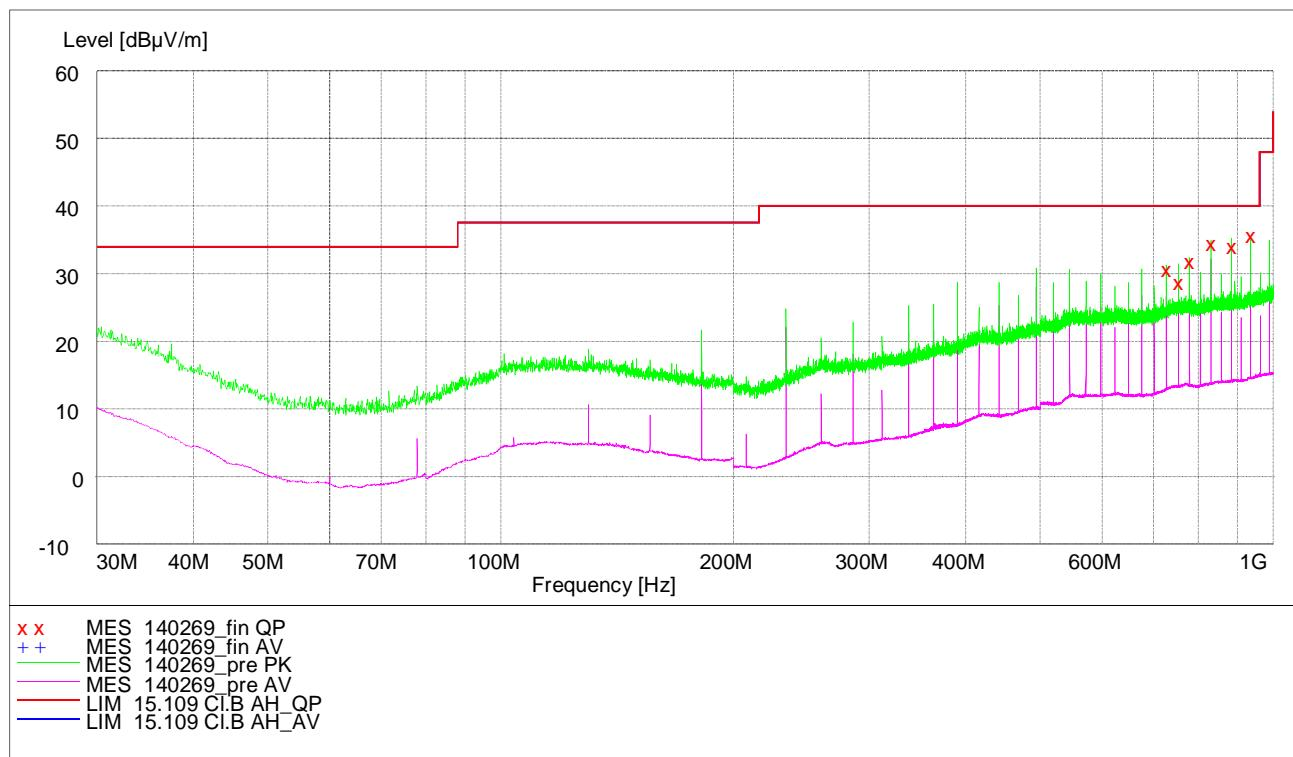
The emissions in the frequency range from 30 MHz to 1 GHz are independent of the set channel. Therefore only measurements at 2441 MHz were carried out.
