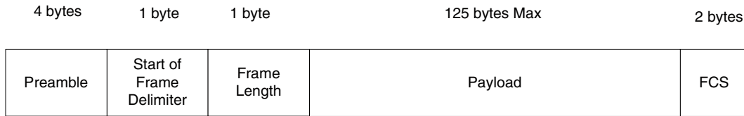
Figure 3. MC13191 Packet Structure
