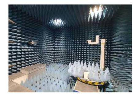
o Size: 5.5(L) m × 5.5(W) m × 5.0(H) m o Frequency range: 700 MHz to 8.0 GHz (Far Field)
