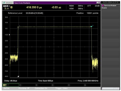
Note 1: Duty Cycle Correction Factor(DCCF) = 20\*log(Duty cycle) = -20.01 dB
