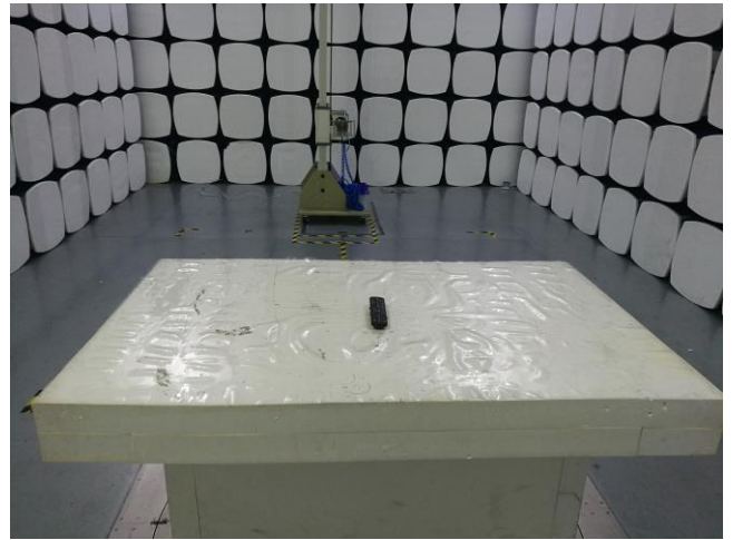
Radiated Emissions Test Setup Above 1GHz
