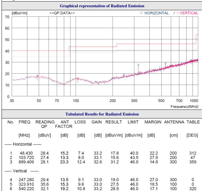
Remark: Margin (dB) = Limit – Result and Result = Reading Peak + Antenna Factor + Loss – Gain Loss and Gain in above table means Cable Loss and Pre-amplifier gain.
