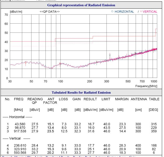
Remark: Margin (dB) = Limit - Result and Result = Reading Peak + Antenna Factor + Loss - Gain
