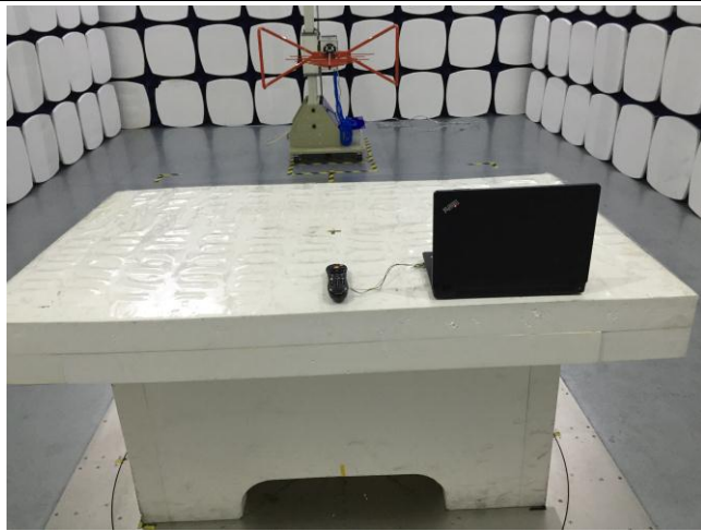
Radiated Spurious Emissions Test Setup Below 1GHz
