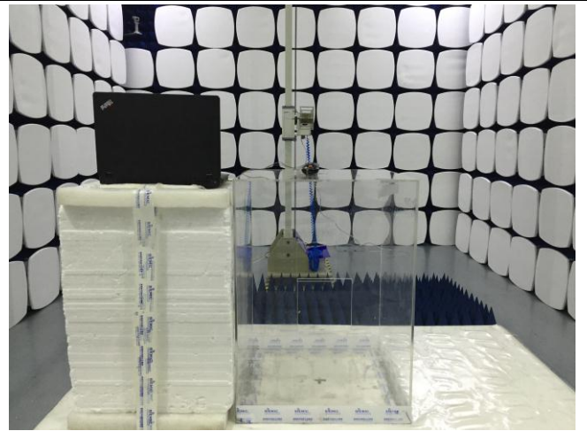
Radiated Spurious Emissions Test Setup Above 1GHz
