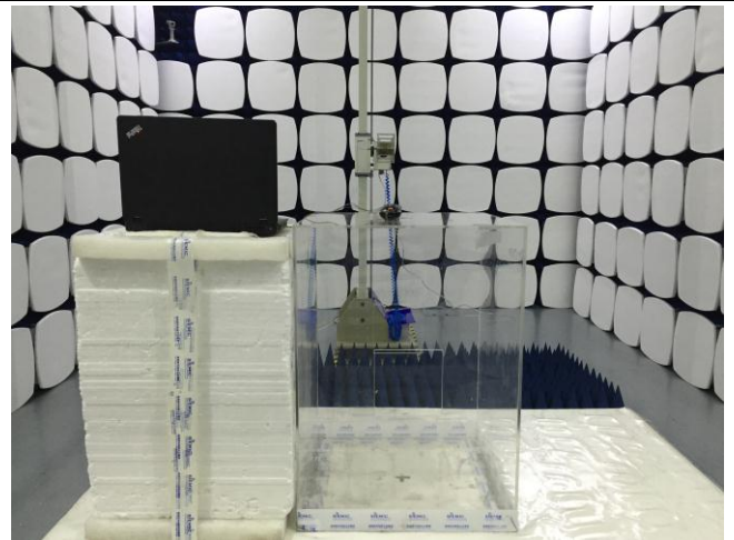
Radiated Spurious Emissions Test Setup Above 1GHz
