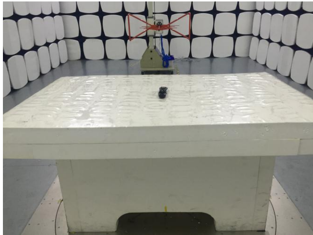
Radiated Emissions Test Setup Below 1GHz
