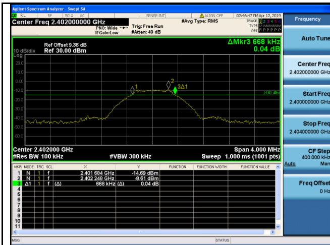
6dB Bandwidth - Low CH 2402
