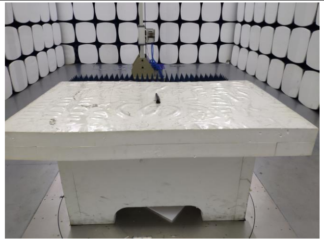
Radiated Emissions Test Setup Above 1GHz
