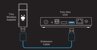
**STEP 3**: If using the extension cable, place the USB adapter on top of your TiVo Mini VOX. For best reception, position the adapter as close as possible to your Wi-Fi router. Use the Velcro to secure the adapter.
