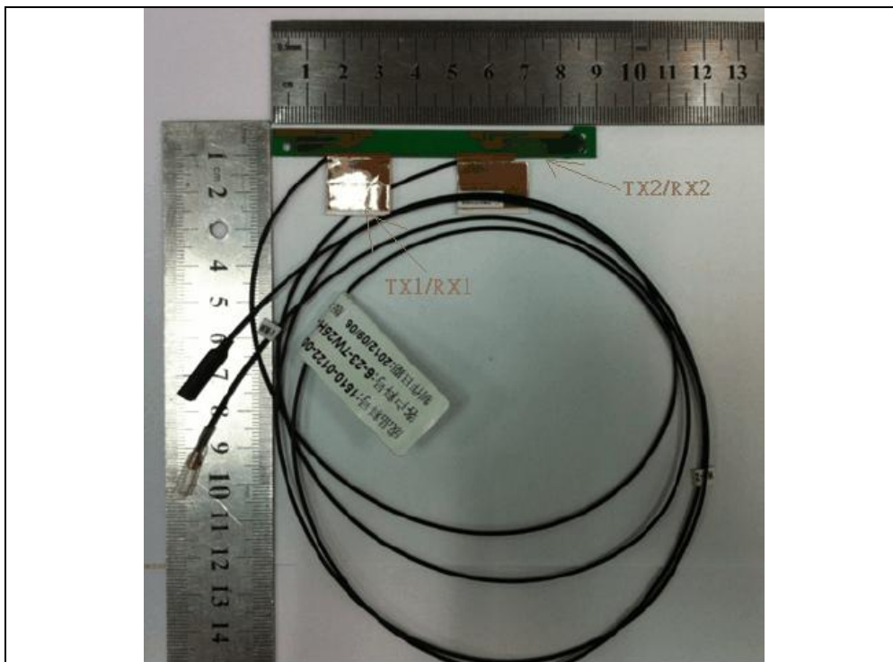
Antenna 5: Brand: FVC / Model: K05007014501(6-23-7W25H-010) (Tx1) & K05007014501(6-23-7W25H-010) (Tx2)
