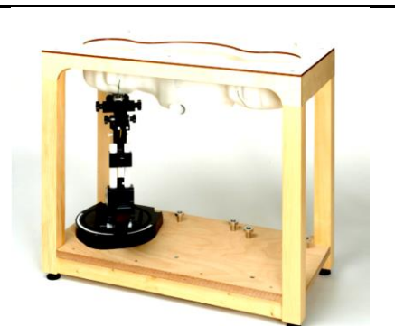
Fig 5.8 Photo of SAM Phantom
