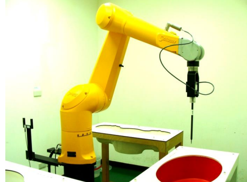
Fig 5.5 Photo of DASY5
