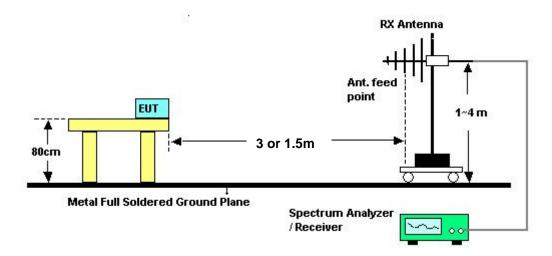
Above 10 GHz shall be extrapolated to the specified distance using an extrapolation factor of 20 dB/decade form 3m to 1.5m.
