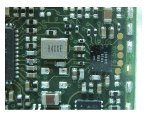
EUT Type 3: Single Port Diversity Transmitter (with one piece splicing by soldering)
