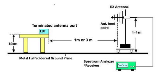
For conducted emissions above 960MHz (Conducted antenna port measurement)
