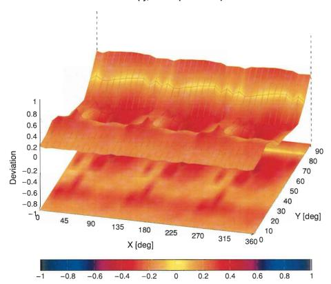
Probe isotropy for E<sub>tot</sub>: probe rotated  $\phi=0^\circ$  to 360°, tilted from field propagation direction  $\vec{k}$  Parallel to the field propagation ( $\psi=0^\circ-90^\circ$ ) at 30 GHz: deviation within  $\pm 0.36$  dB Parallel to the field propagation ( $\psi=0^\circ-90^\circ$ ) at 60 GHz: deviation within  $\pm 0.45$  dB
