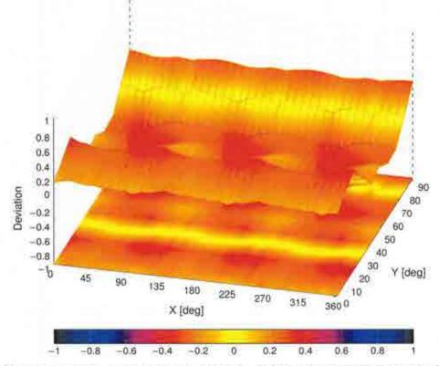
Probe isotropy for E<sub>tot</sub>: probe rotated  $\phi = 0^{\circ}$  to 360°, tilted from field propagation direction  $\vec{k}$ Parallel to the field propagation ( $\psi = 0^{\circ} - 90^{\circ}$ ) at 30 GHz: deviation within ±0.32 dB Parallel to the field propagation ( $\psi = 0^{\circ} - 90^{\circ}$ ) at 60 GHz: deviation within ±0.44 dB
