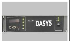
The DASY5 measurement server is based on a PC/104 CPU board with a 166MHz low-power Pentium, 32MB chip disk and 64MB RAM. The necessary circuits for communication with either the DAE4 electronic box as well as the 16-bit AD-converter system for optical detection and digital I/O interface are contained on the DASY5 I/O-board, which is directly connected to the PC/104 bus of the CPU board.
