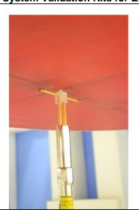
Construction: Symmetrical dipole with 1/4 balun **Enables**
