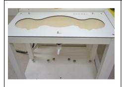
Construction: The shell corresponds to the specifications of the Specific Anthropomorphic Mannequin (SAM) phantom defined in IEEE1528: 2013. It enables the dosimetric evaluation of left and right hand phone usage as well as body mounted usage at the flat phantom region. A cover prevents evaporation of the liquid. Reference markings on the phantom allow the complete setup of all predefined phantom positions and measurement grids by manually teaching three points with the robot.
