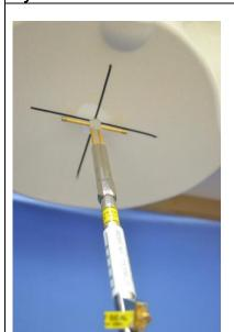
Construction: Symmetrical dipole
