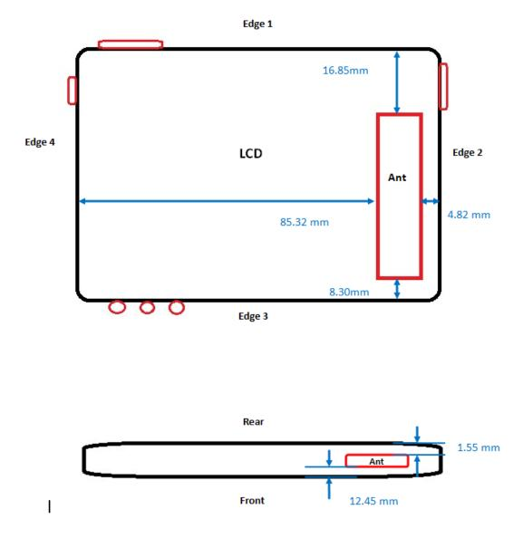
9.1.1 SAR Required Test Configuration
