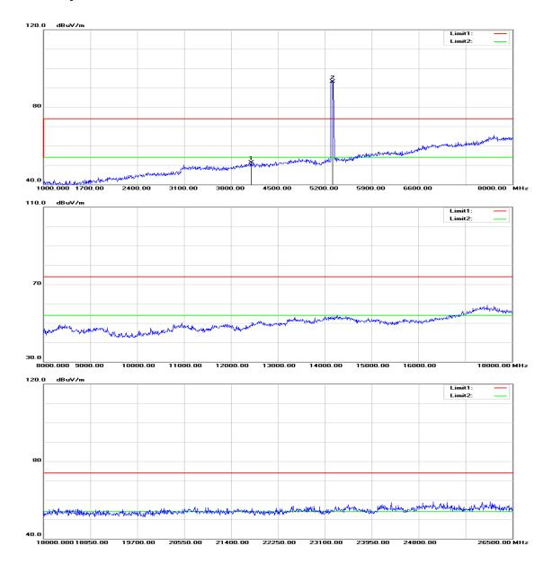
Operation Mode: Tx / IEEE 802.11n HT 40 MHz mode / 5310 Test Date: July 31, 2015
