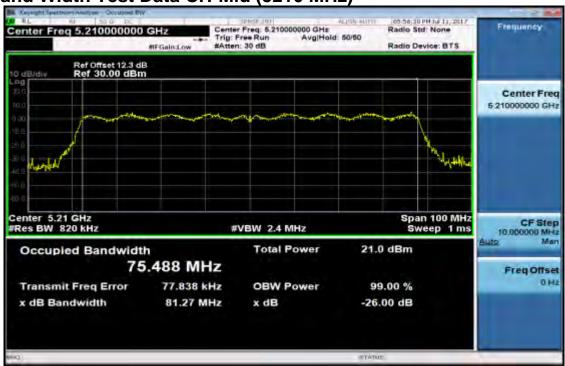
802.11ac VHT80, 5150~5250 MHz (Aux) 26dB Band Width Test Data CH-Mid (5210 MHz)
