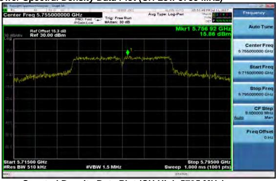
Peak Power Spectral Density Data Plot (CH High 5795 MHz)
