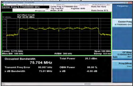
802.11ac VHT80, 5725~5850 MHz (Aux) 6dB Band Width Test Data CH-Low (5775 MHz)
