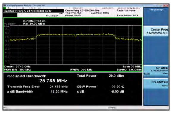
6dB Band Width Test Data CH-Mid (5785 MHz)
