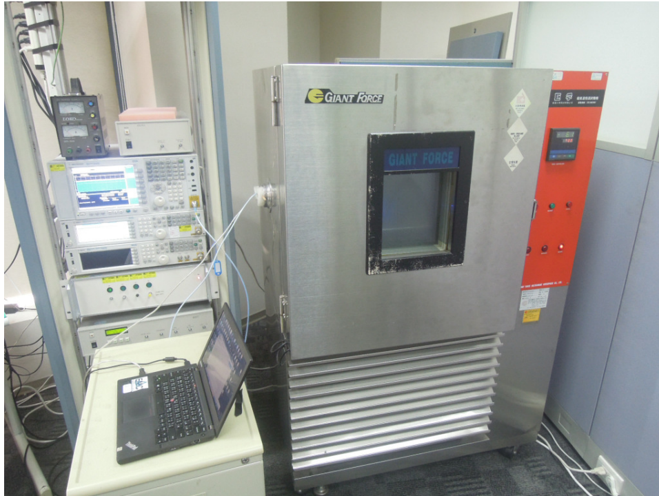
Photograph 5: Set-up for Conducted testing
