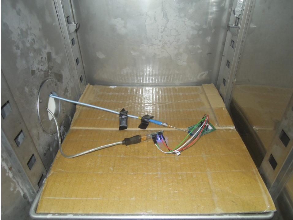
Photograph 6: Set-up for Conducted testing
