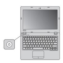
**Note:** To prevent over-discharging, the battery pack of the computer is placed in Ship Mode at the factory. While the battery is in Ship Mode, it will not provide power to the computer. Connect your computer to the supplied AC power adapter before first use. The battery pack will be activated instantly when the computer is connected to AC power.
