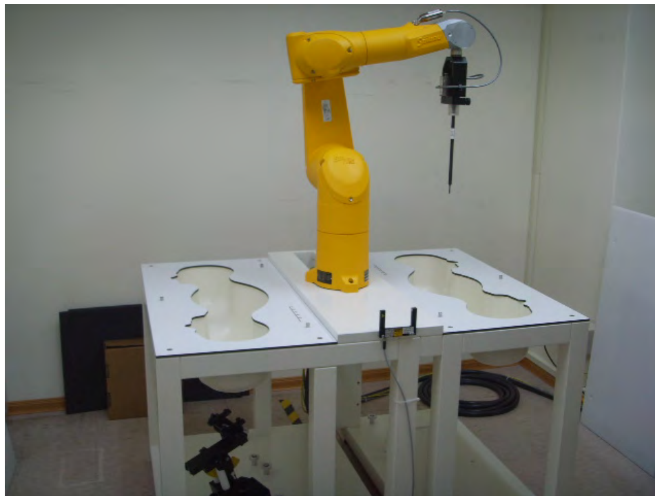
Fig.1 Photograph of the SAR measurement system
