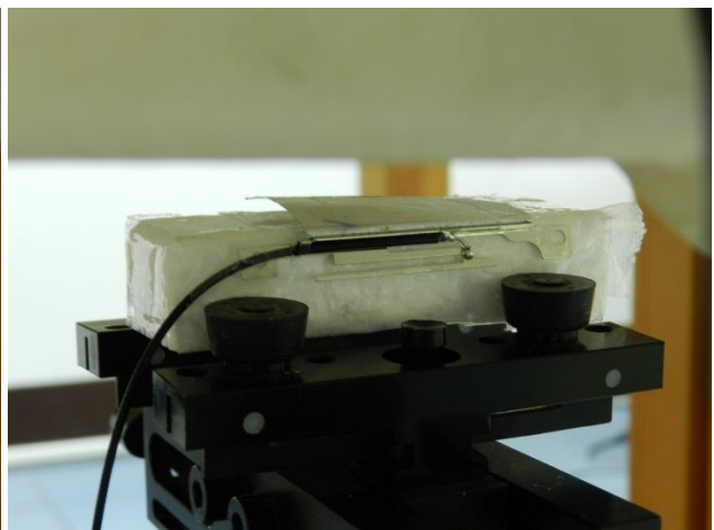
Bottom Side of the DUT with Phantom 1.7 cm Gap
