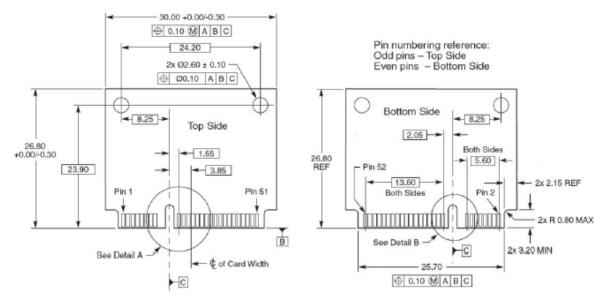
Figure 1. RTL8192CE miniCard Mechanical Specification
