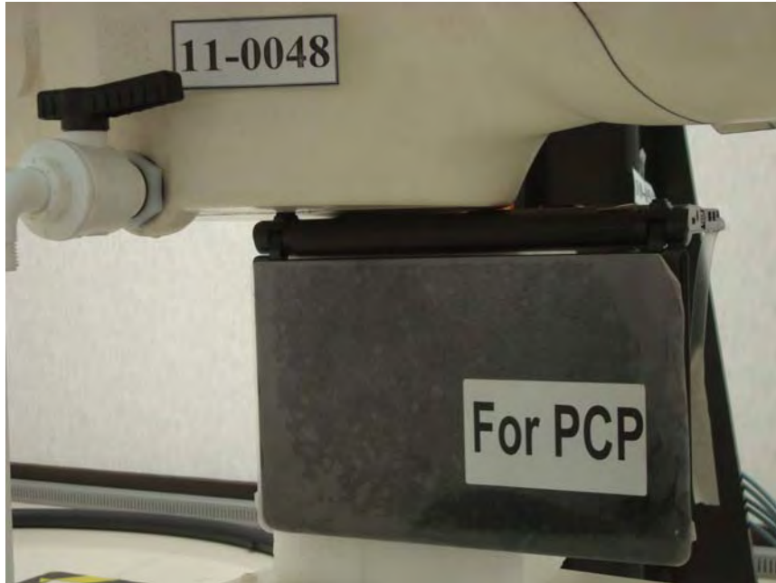
Figure 1. Body SAR Test Setup (Flat Section) Host: LCD Open 90° Bottom Close Body
