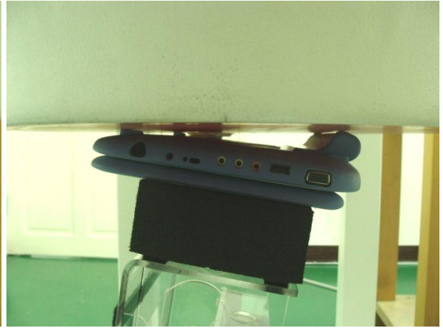
Fig 9.5 Bottom of Tablet Touching with 0 cm Air Gap (DUT with Battery 2)
