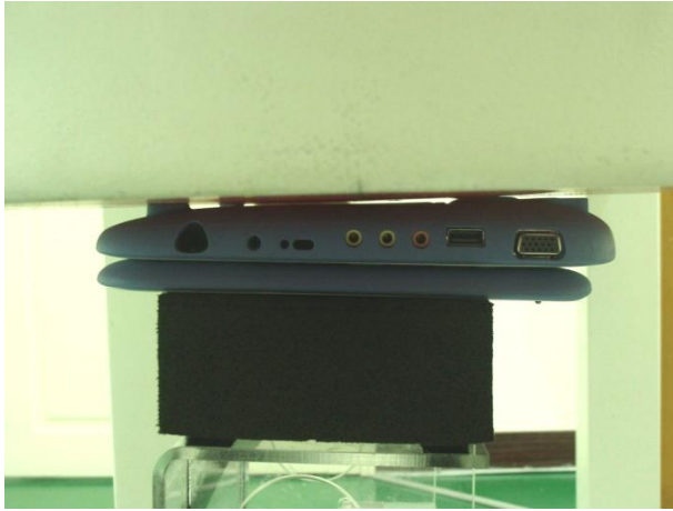
Fig 9.4 Bottom of Tablet Touching with 0 cm Air Gap (DUT with Battery 1)
