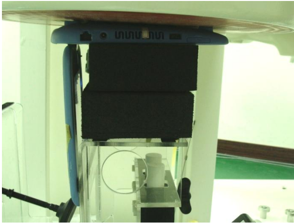
Fig 9.1 Bottom of Laptop Touching with 0 cm Air Gap (DUT with Battery 1)
