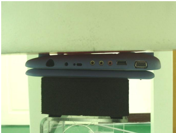
Fig 9.6 Bottom of Tablet Touching with 0 cm Air Gap (DUT with Battery 3)
