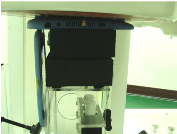
Fig 9.3 Bottom of Laptop Touching with 0 cm Air Gap (DUT with Battery 3)
