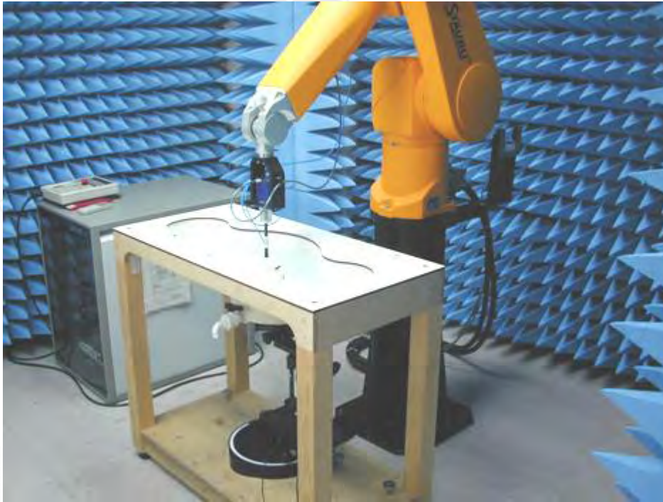
Fig.1 Photograph of the SAR measurement System
