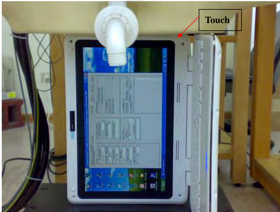
Fig.5 Right side of EUT is paralleled with flat phantom, Right side is contact with flat phantom.
